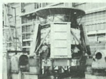
Apollo Telescope Mount during vibration testing
