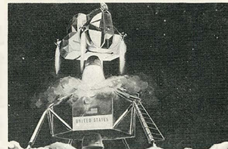
With descent stage as a launch pad, the ascent stage fires for liftoff.
