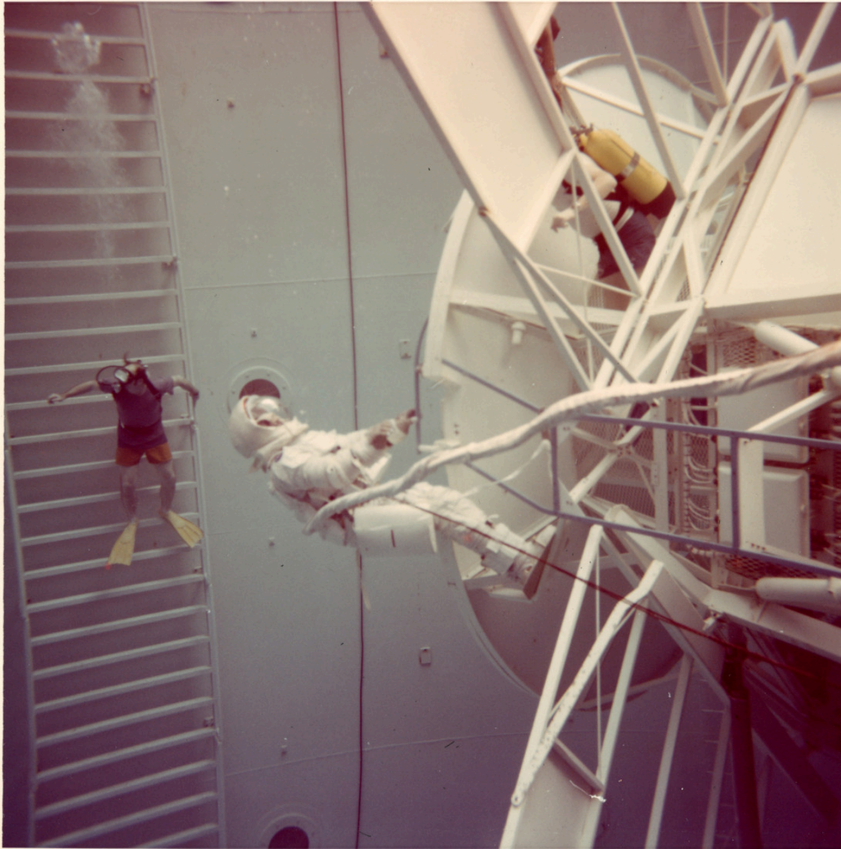
There is a still caption on the back which reads: "NEUTRAL BUOYANCY SKYLAB EVA TRAINING, ASTRONAUT KERWIN (EV2) WITH FEET SECURED IN FOOT RESTRAINTS AT ATM SUN-END TRANSFER STATION."
