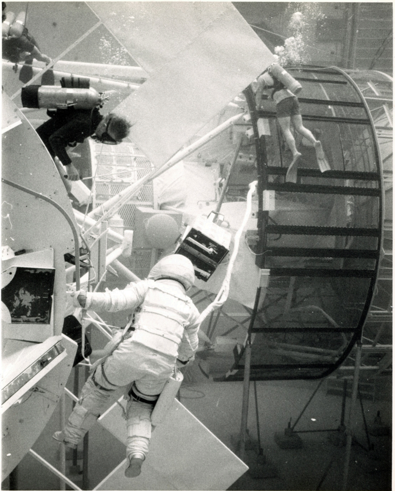
There is a still caption on the back which reads: "NEUTRAL BUOYANCY, ASTRONAUT SCHWEICKART AT FAS WORK STATION EXTENDING BOOM WITH FILM MAGAZINE TO ATM."
