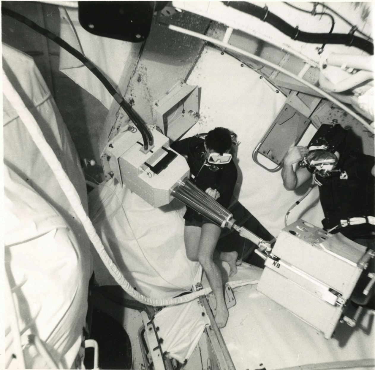
There is a still caption on the back which reads: "NEUTRAL BUOYANCY, ASTRONAUT MUSGRAVE AT ATM SUN-END RECEIVING FILM MAGAZINE FROM FAS ON EXTENDABLE BOOM."
