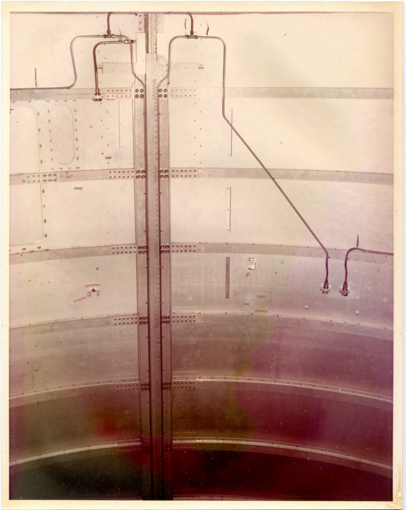
There is a still caption on the back which reads: "Airlock payload shroud. Detail separation rail position I. March 1971 Input."
