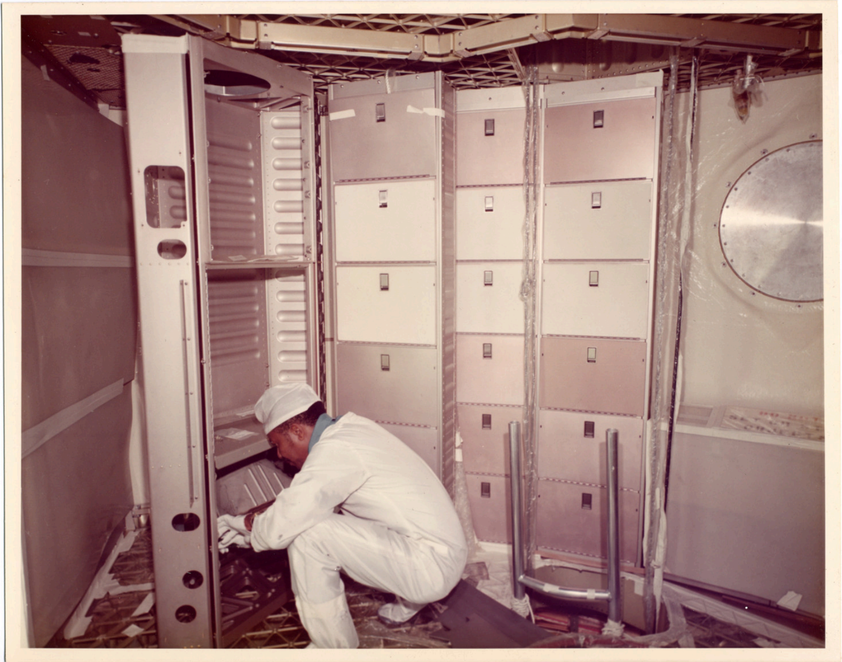
There is a still caption on the back which reads: "INSTALLING BOTTOM PANEL IN STORAGE CABINET IN WARDROOM OWS-1 SEPT 1971 INPUT."
