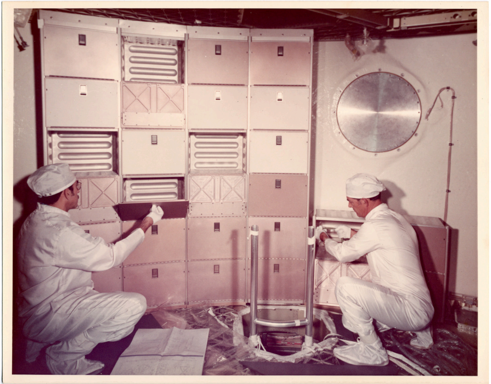
There is a still caption on the back which reads: "COMPLETING INSTALLATION OF STOWAGE LOCKERS & DATA FILE UNDER OBSERVATION WINDOW, OWS-1 INPUT FOR SEPT 1971"
