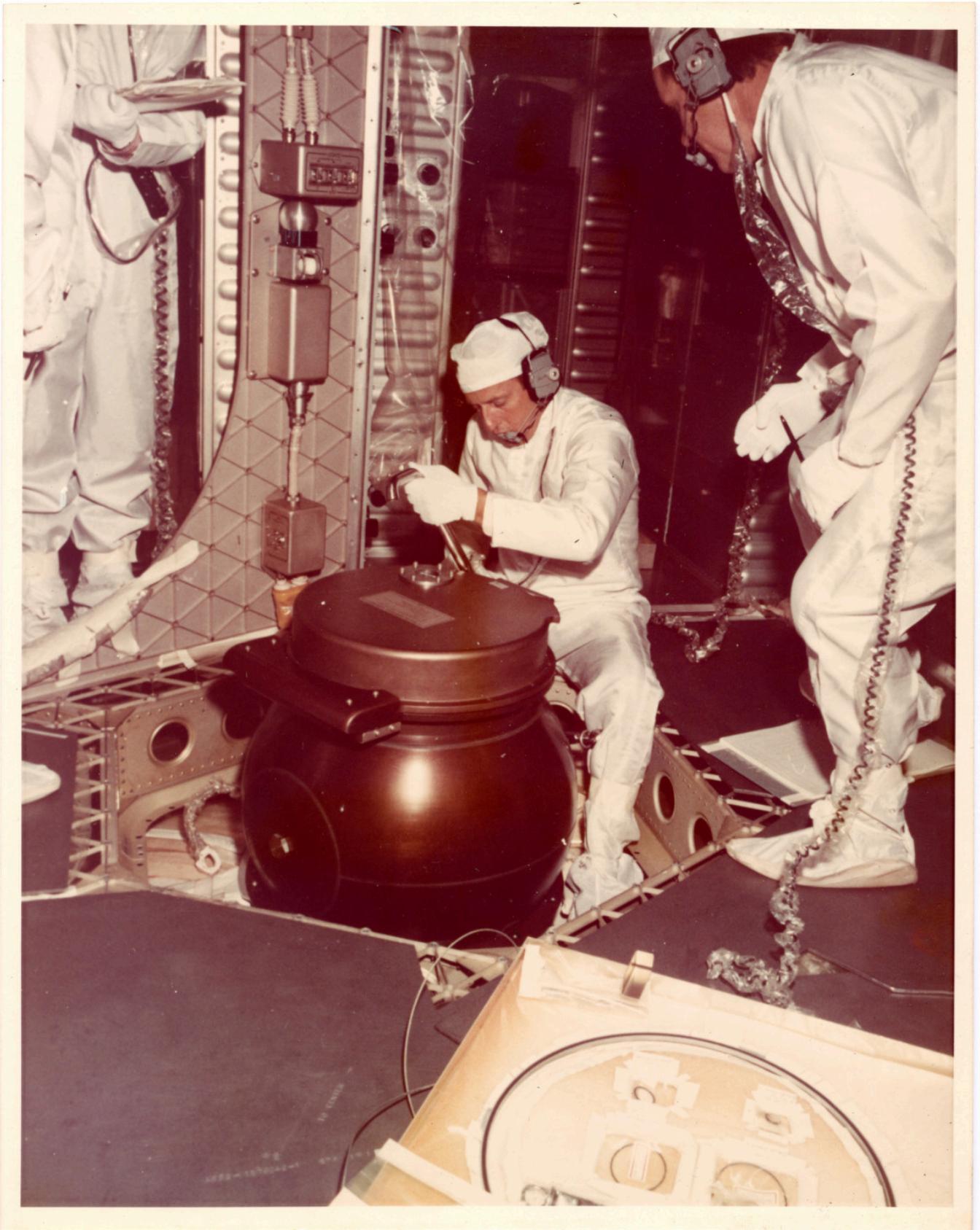
There is a still caption on the back which reads: "ASTRONAUT CONRAD CLOSING TRASH DISPOSAL AIRLOCK. OWS NO-1."
