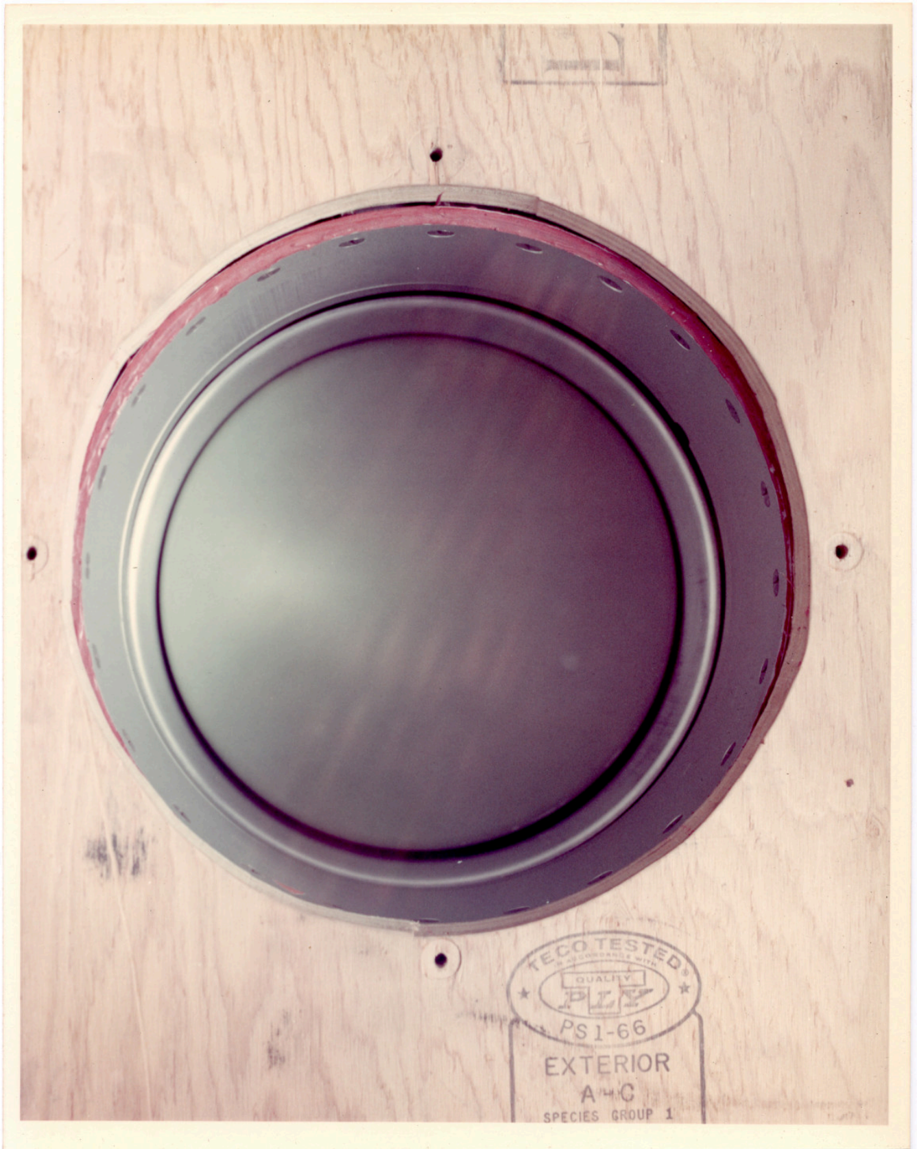
There is a still caption on the back which reads: "EJECTION PLATE INSIDE THE TRASH DISPOSAL AIRLOCK WITH OUTBOARD HATCH IN OPEN POSITION. OWS INPUT FOR SEPT 1971."
