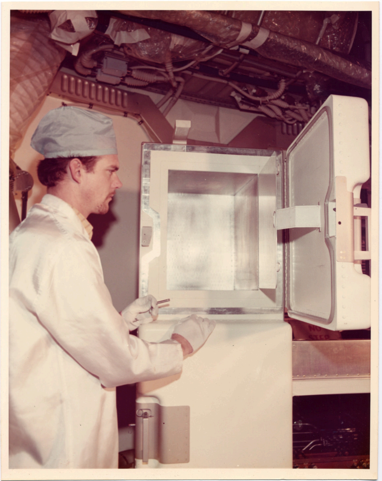
There is a still caption on the back which reads: "CLOSE UP OF FOOD FREEZER IN UPPER LEVEL. OWS NO. 1"
