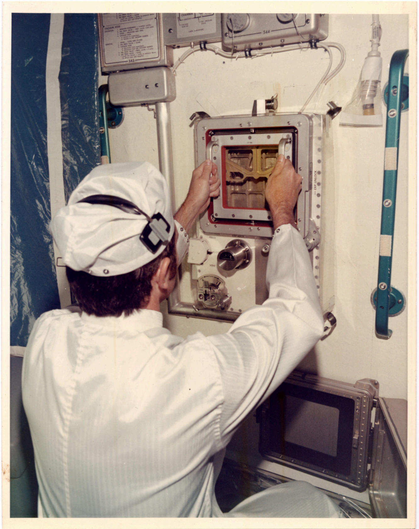
There is a still caption on the back which reads: "ASTRONAUT TRULY PLACING WINDOW UNIT IN SCIENTIFIC AIRLOCK. OWS NO-1."
