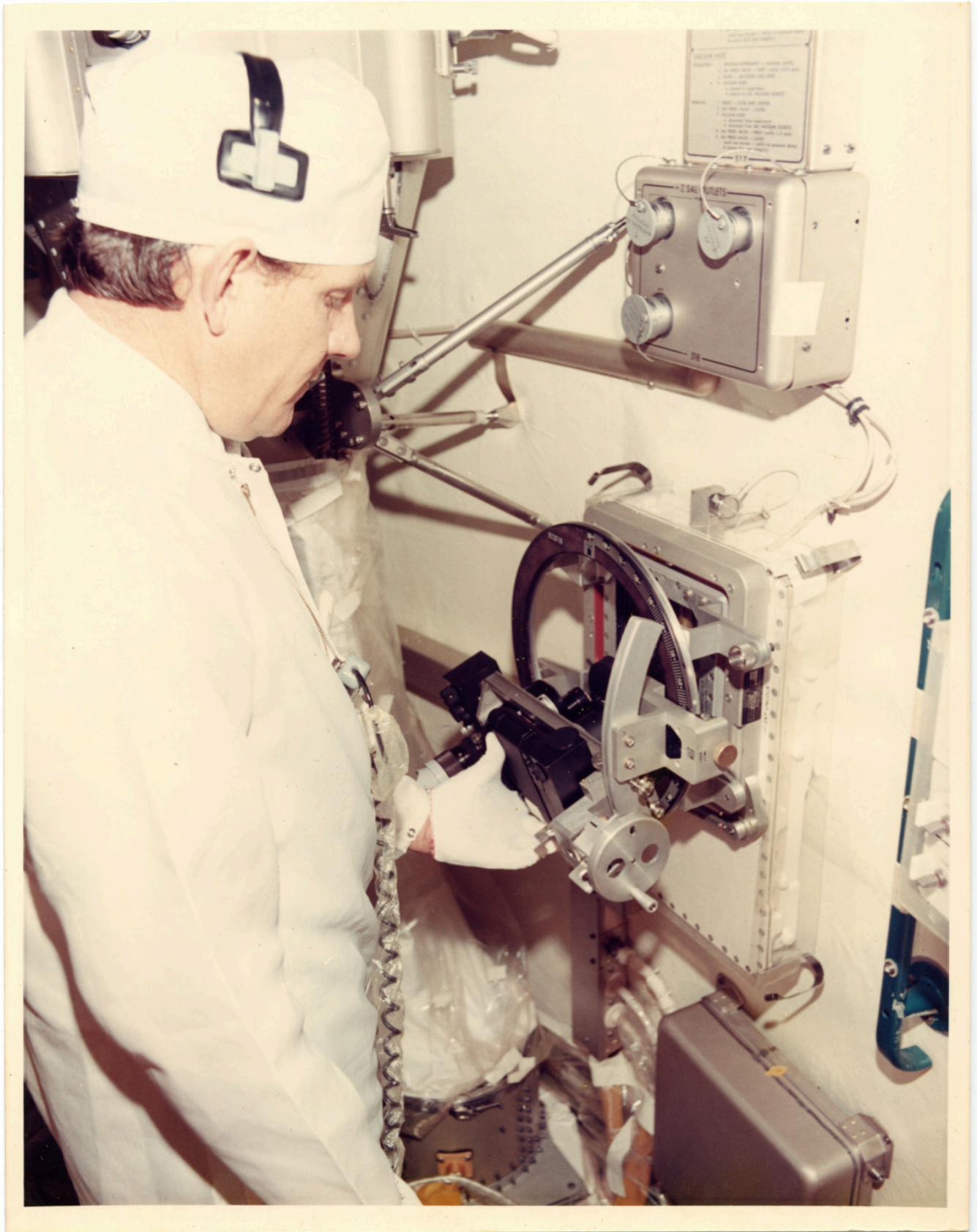
There is a still caption on the back which reads: "CHECKING OUT TO-63 CAMERA ASSEMBLY MOUNTED IN OWS NO-1 SCIENTIFIC AIRLOCK"
