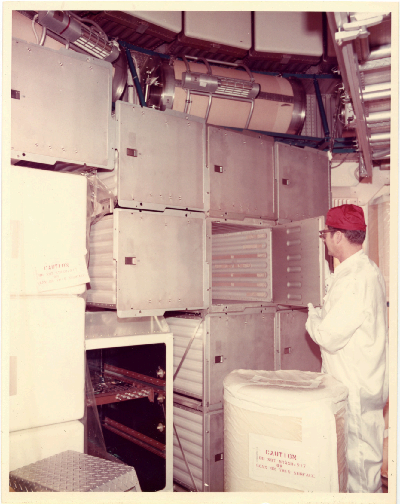
There is a still caption on the back which reads: "STOWAGE RACKS BEING INSPECTED AFTER PRE-FIT CHECKOUT. OWS NO-1."
