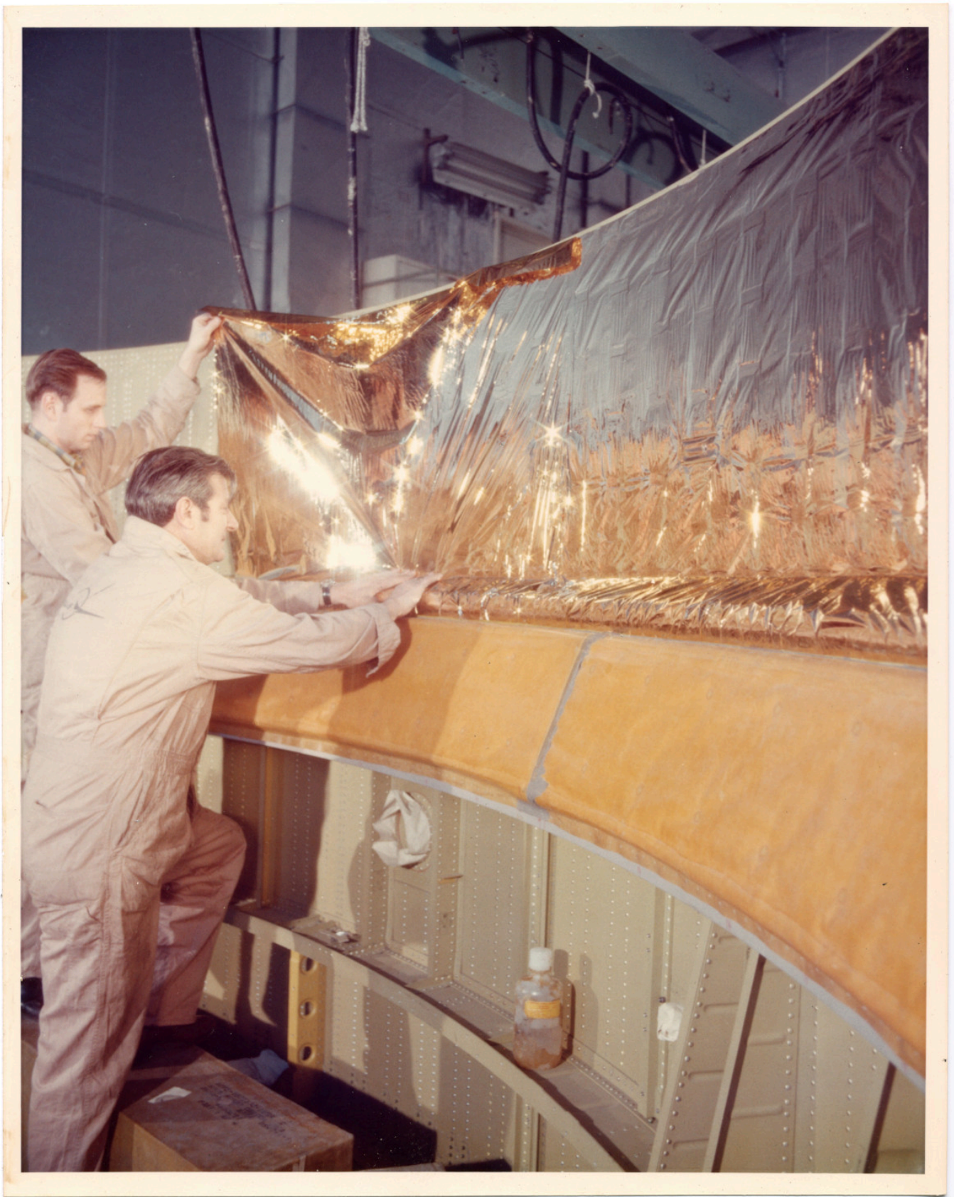
There is a still caption on the back which reads: "BONDING GOLD FOIL TO AFT SKIRT OF OWS BACKUP VEHICLE."
