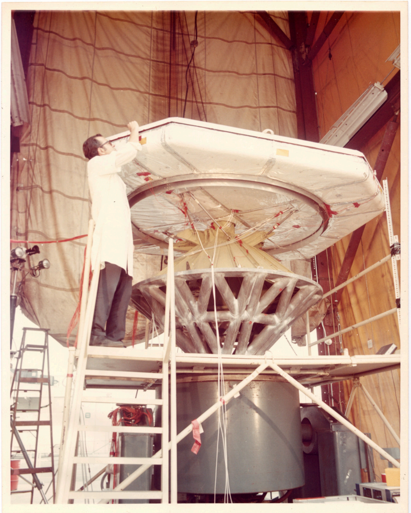
There is a still caption on the back which reads: "MAKING FINAL CHECK OF INSTRUMENTATION LEAD OF OWS RADIATOR PRIOR TO VIBRATION TESTING."
