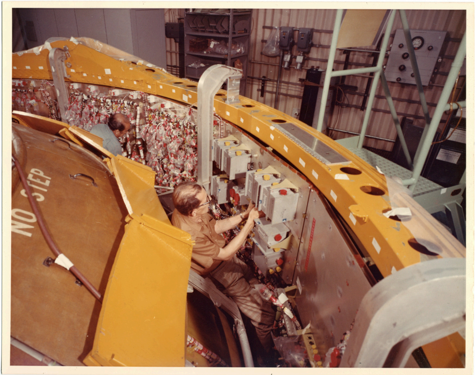
There is a still caption on the back which reads: "INSTALLING ELECTRICAL HARNESSSES ON FORWARD SKIRT OF OWS #1, AUG. 1971 INPUT."
