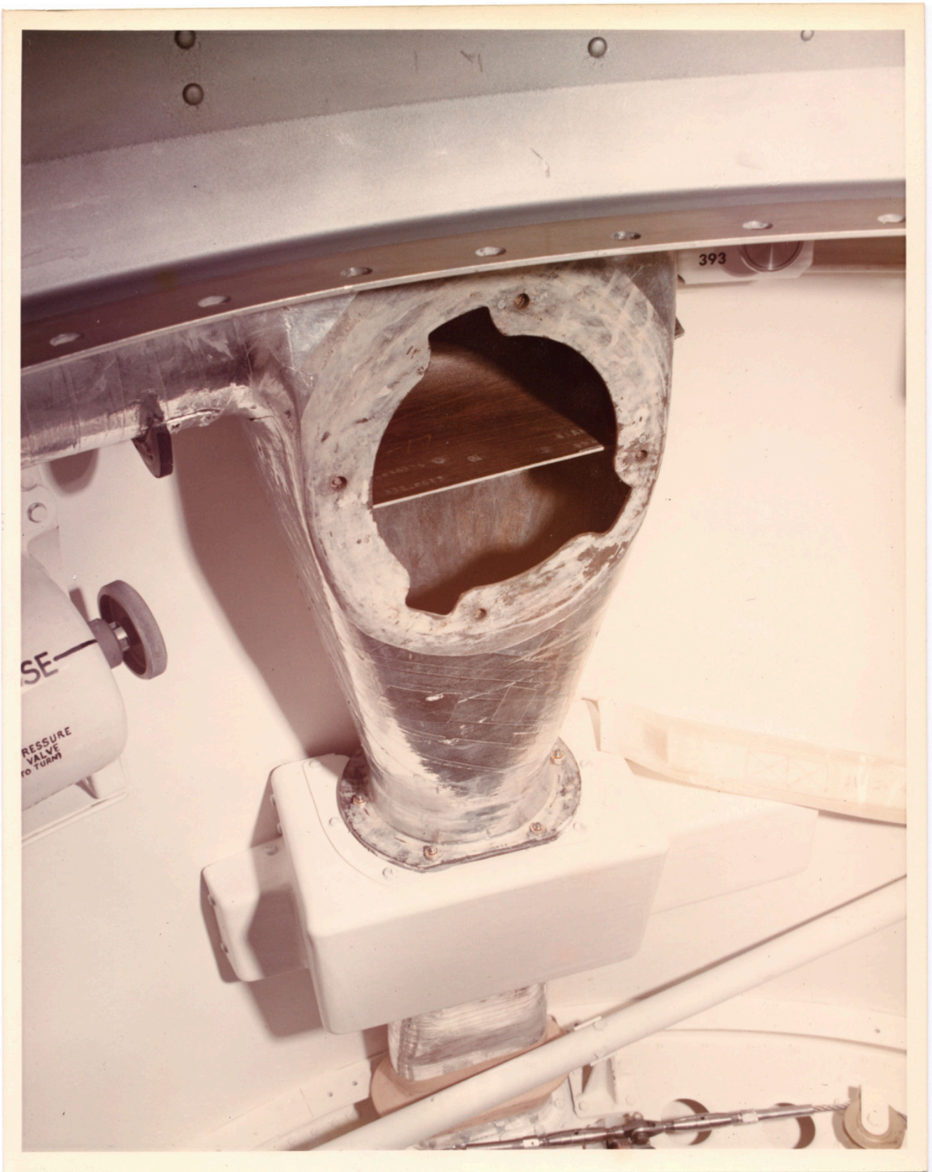
There is a still caption on the back which reads: "Airlock zone 4 closeup of end of OWS supply duct open. MDAC Input for June."
