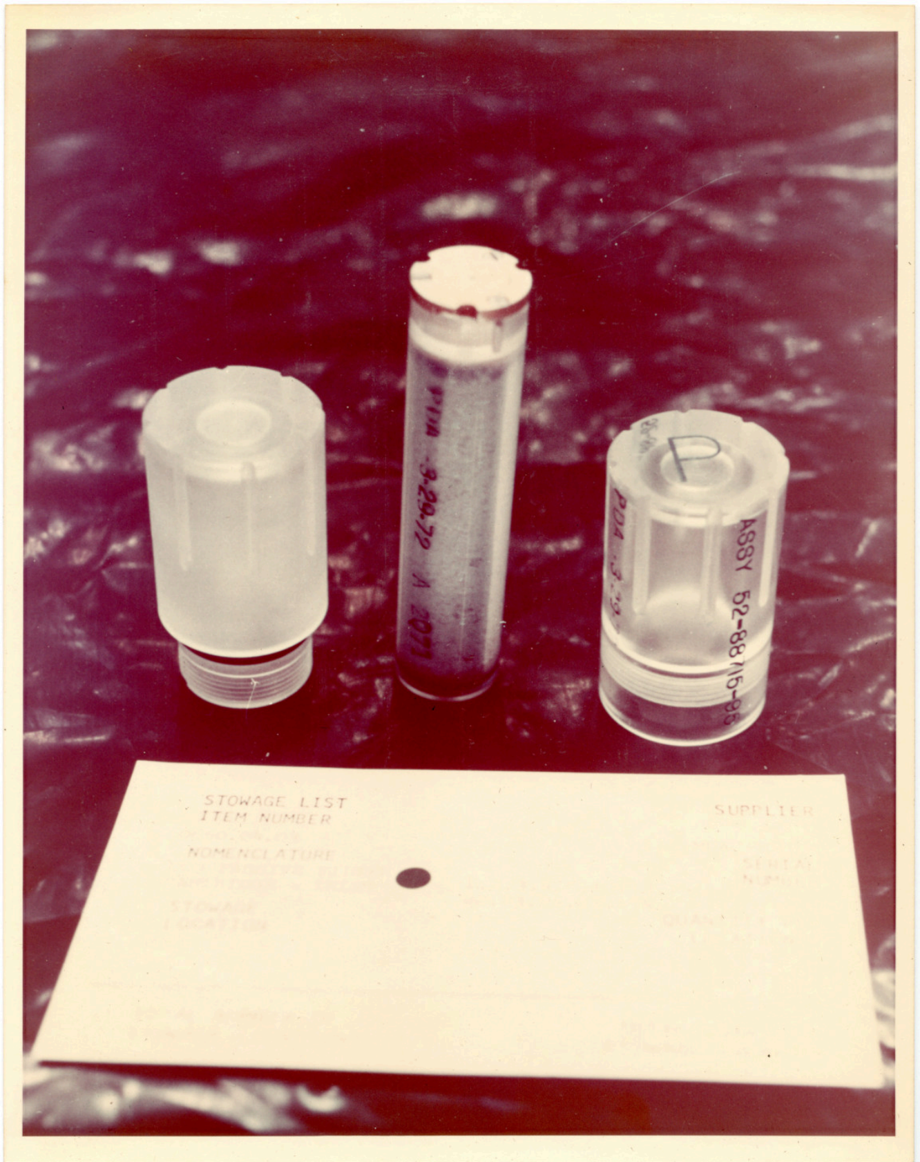
There is a still caption on the back which reads: "Airlock zone 1&2 passive PPCO2 filter cartridge MDAC Input for June"
