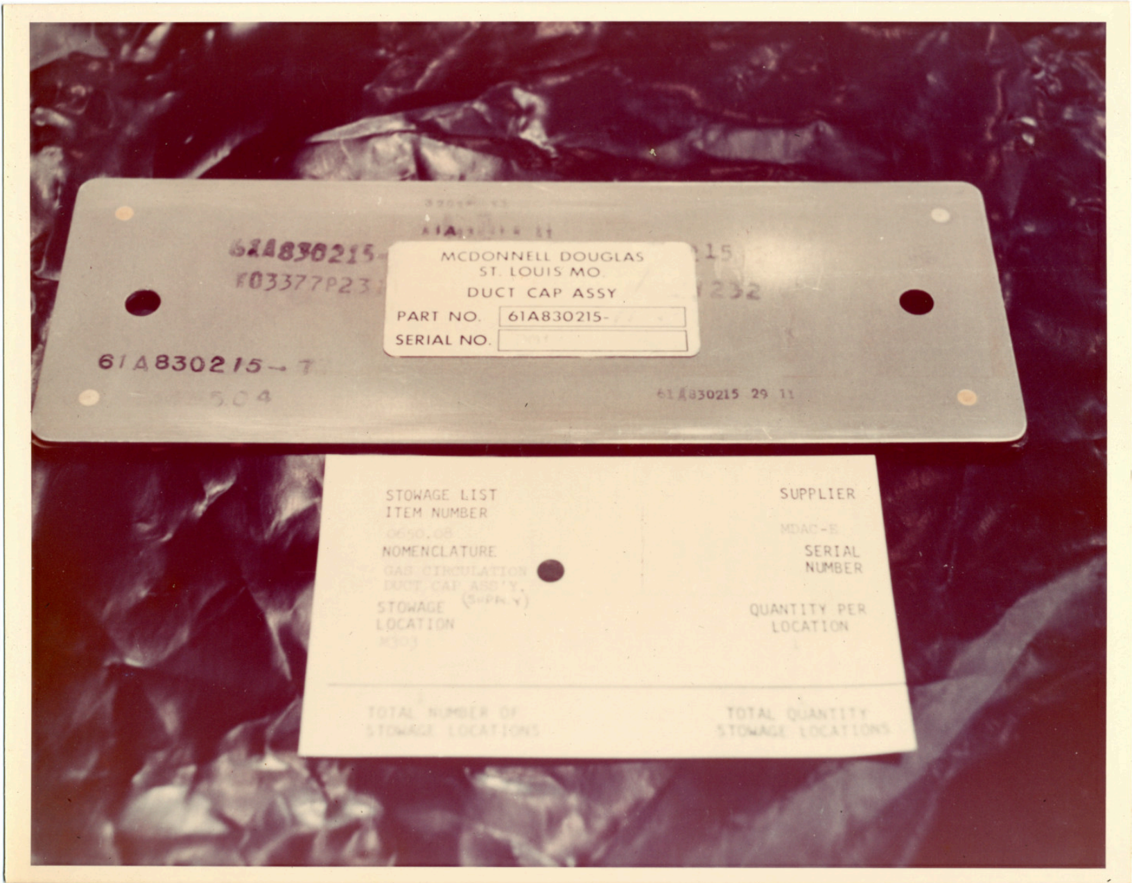
There is a still caption on the back which reads: "Airlock zone 2 gas circulation duct cap assembly MDAC Input for June"
