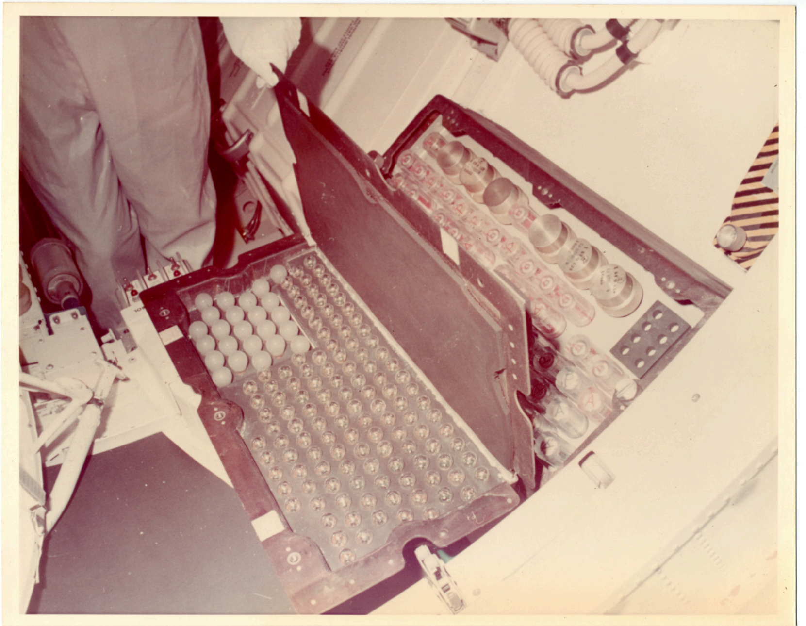
There is a still caption on the back which reads: "Airlock Flight Article #1 in clean room closeup of stowage container MDAC Input for Aug"
