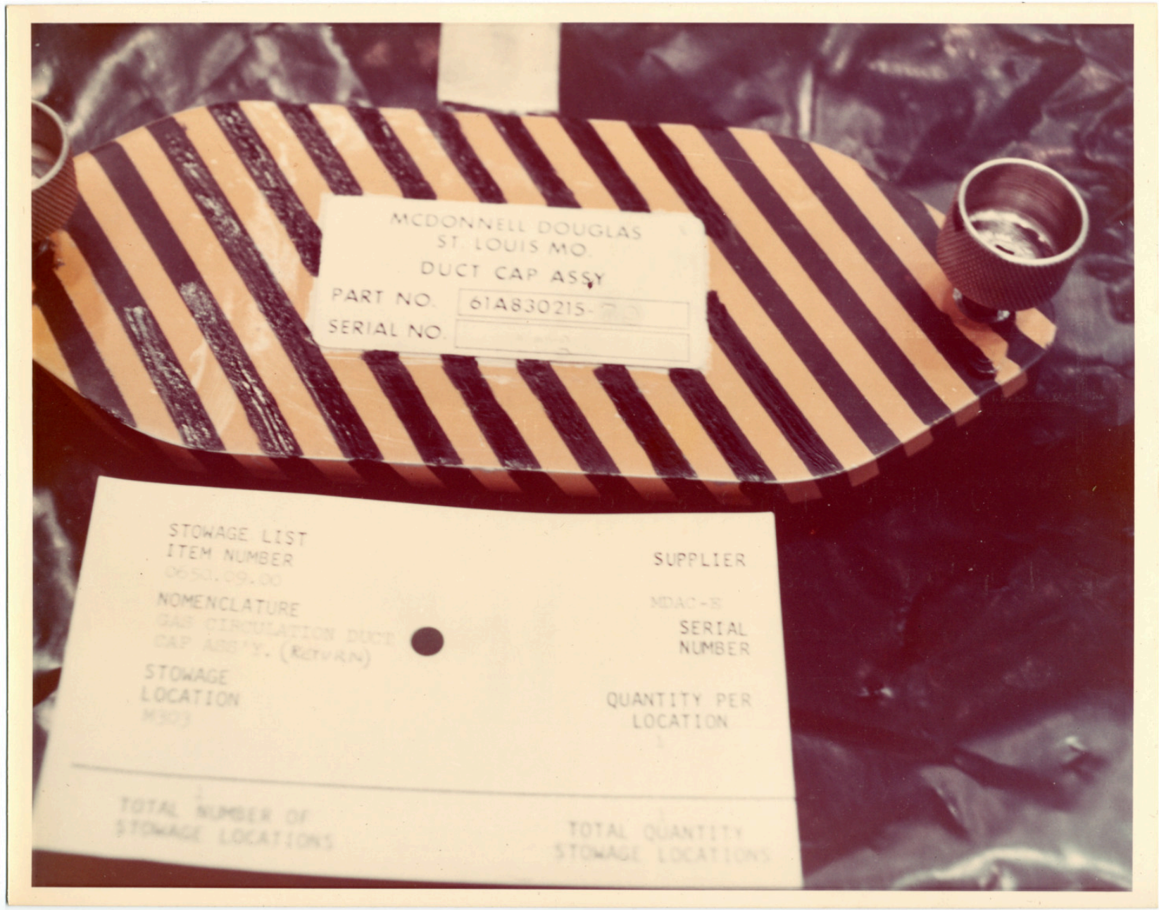
There is a still caption on the back which reads: "Airlock zone 2 sas circulated duct cap assembly. MDAC Input for June."
