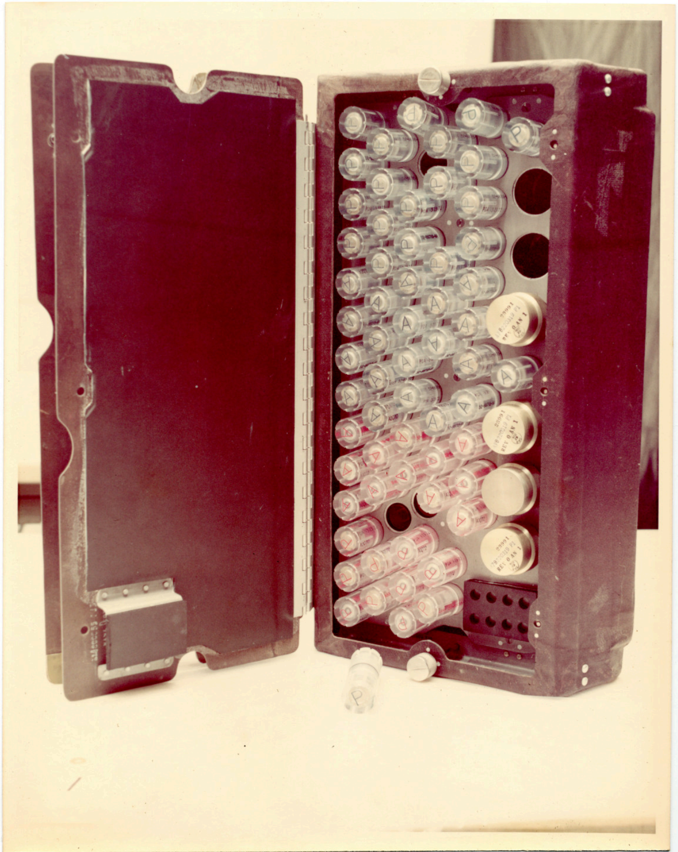
There is a still caption on the back which reads: "Airlock zone 2 PPCO2 filter cartridge. MDAC Input for June."
