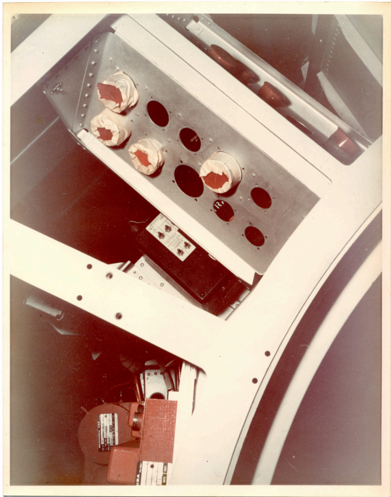
There is a still caption on the back which reads: "NASA TRAINER-EXTERIOR OF STS SHOWING MDA INTERFACE CONNECTORS AND SEQUENTIAL POWER CONTROL PANEL, AND COOLANOL 15 RESERVOIRS. NASA-1567"
