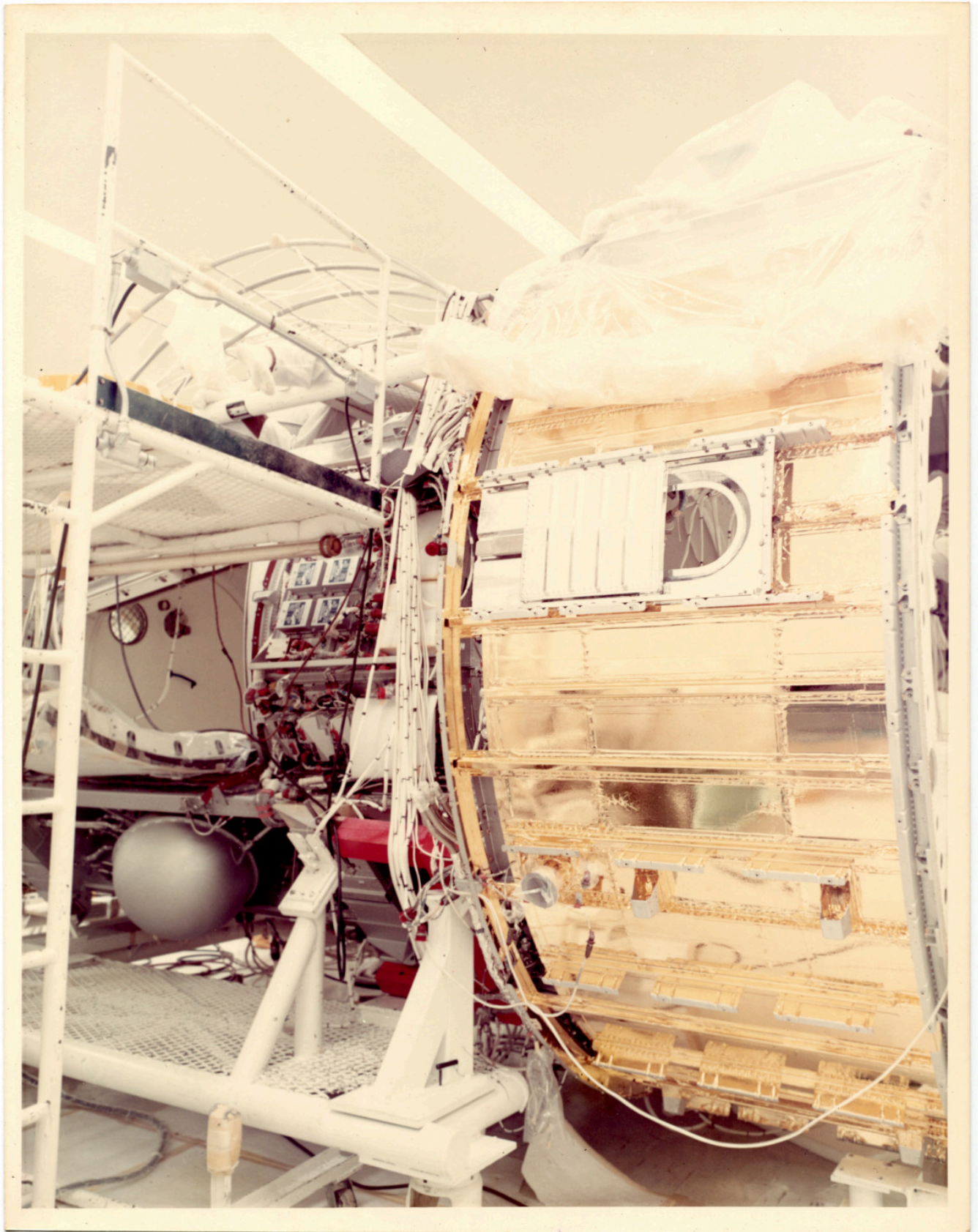
There is a still caption on the back which reads: "AIRLOCK FLIGHT ARTICLE NO. 1 IN CLEAN ROOM AT MDAC-E BLDG. 101-3/4 VIEW LOOKING AFT SHOWING ELECTRONIC MODULE #1 AND #4 CT-15. NASA-1363"
