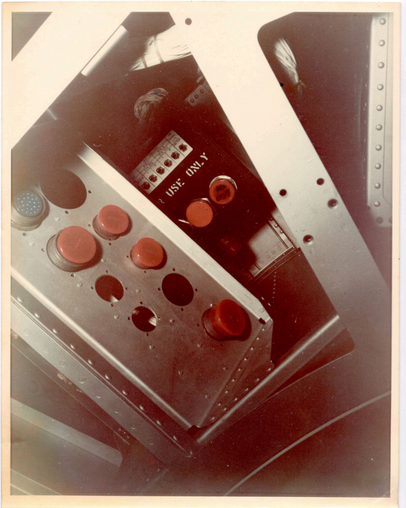
There is a still caption on the back which reads: "NASA TRAINER - EXTERIOR OF STS SHOWING MDA INTERFACE CONNECTIONS AND SEQUENTIAL POWER CONTROL PANEL. NASA-1566."
