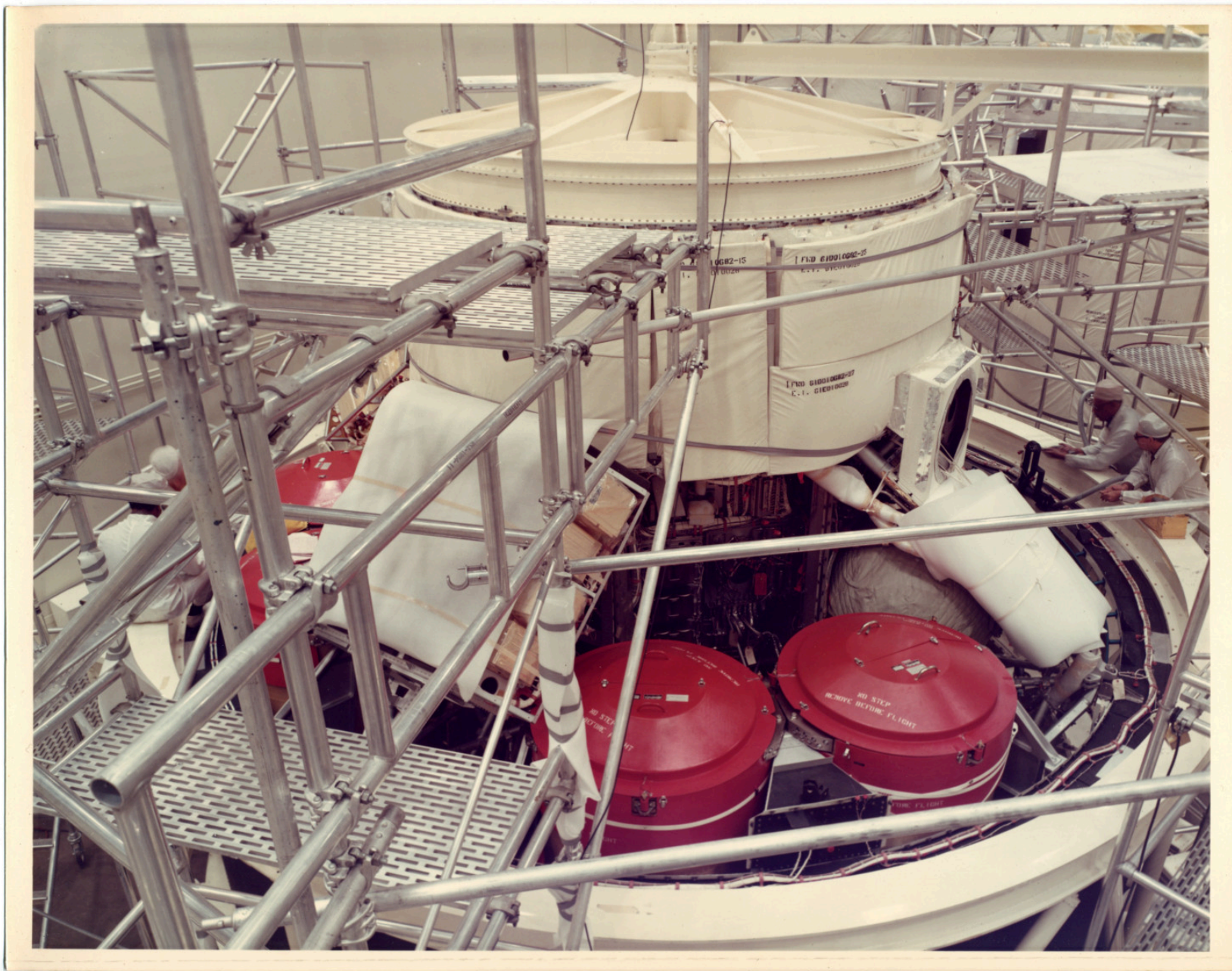
There is a still caption on the back which reads: "AIRLOCK FLIGHT ARTICLE NO. 1 IN CLEAN ROOM. MATE AND ALIGNMENT OF FAS/AM."
