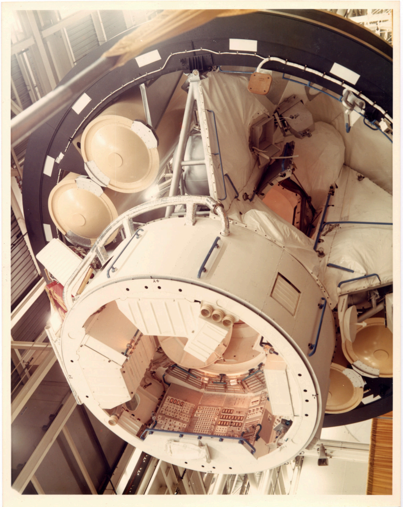
There is a still caption on the back which reads: "AIRLOCK NASA TRAINER ON PRODUCTION LINE IN MDAC-E BLDG-101 /3/4 VIEWLOOKING AFT SHOWING STS CONTROL & CIRCUIT BREAKER PANELS INTERIOR, O2 TANKS & EVA AREA."
