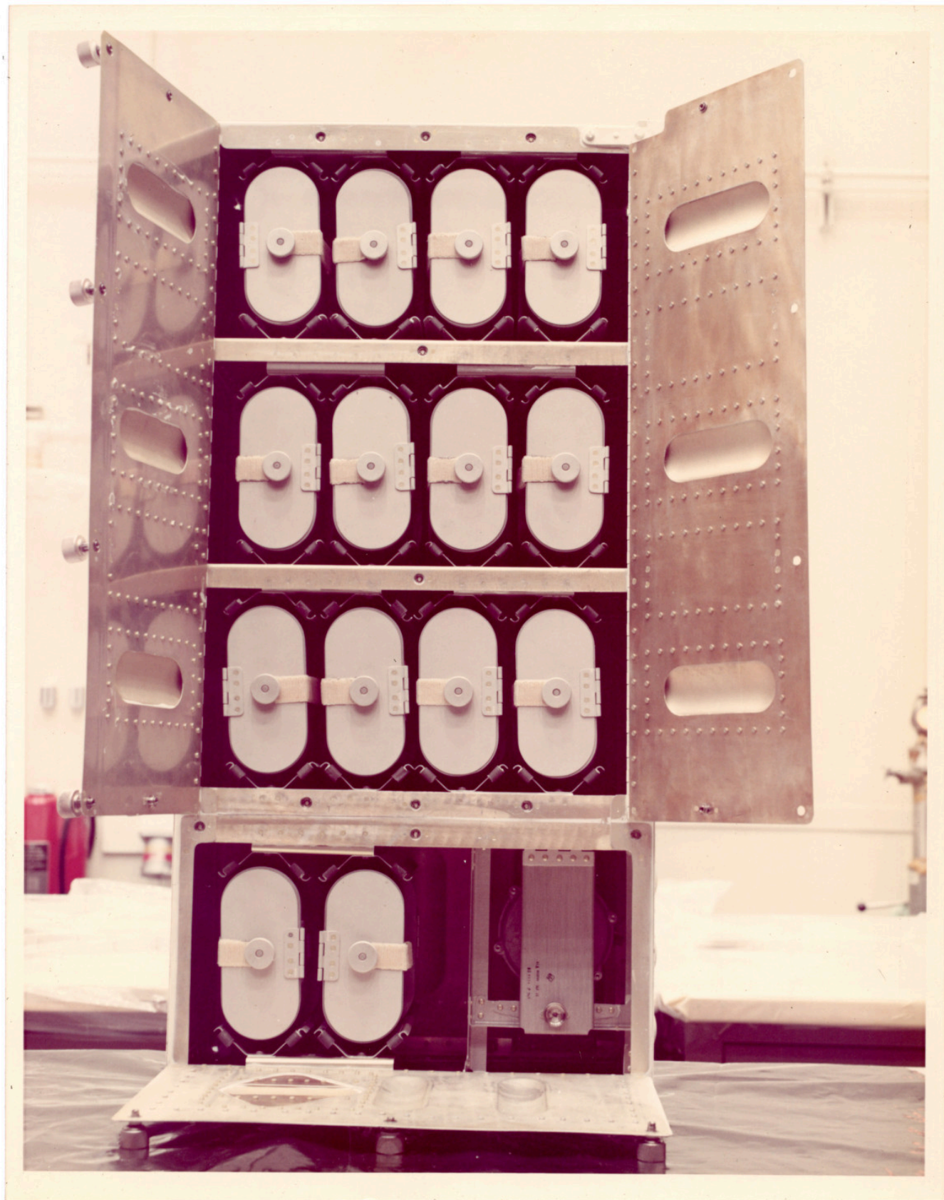
There is a still caption on the back which reads: "Airlock zone 1 stowage container. MDAC Input for June."
