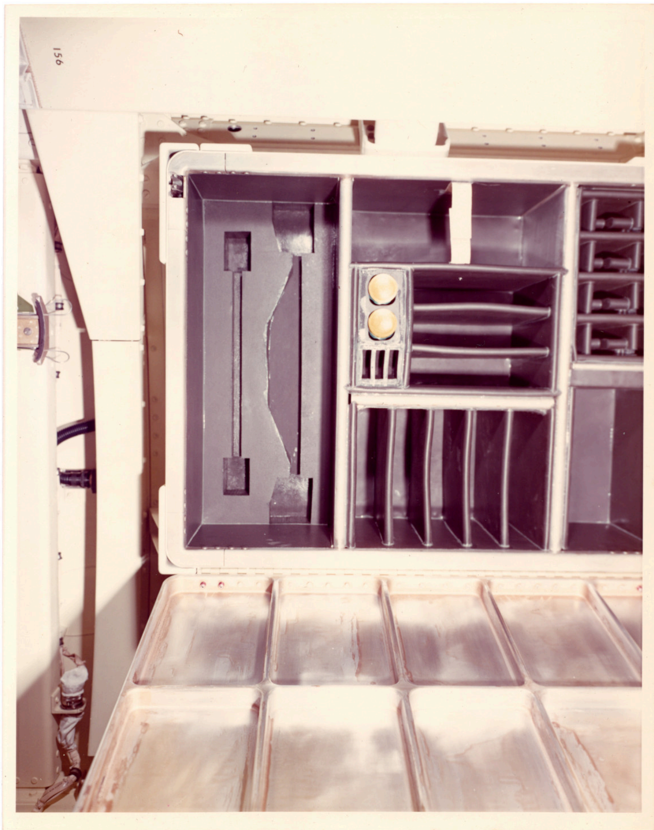
There is a still caption on the back which reads: "MOSITE CUTOUTS AS INSTALLED IN THE MISCELLANEOUS STOWAGE CONTAINER OF MDA BACKUP ARTICLE. MDAC INPUT FOR AUGUST."
