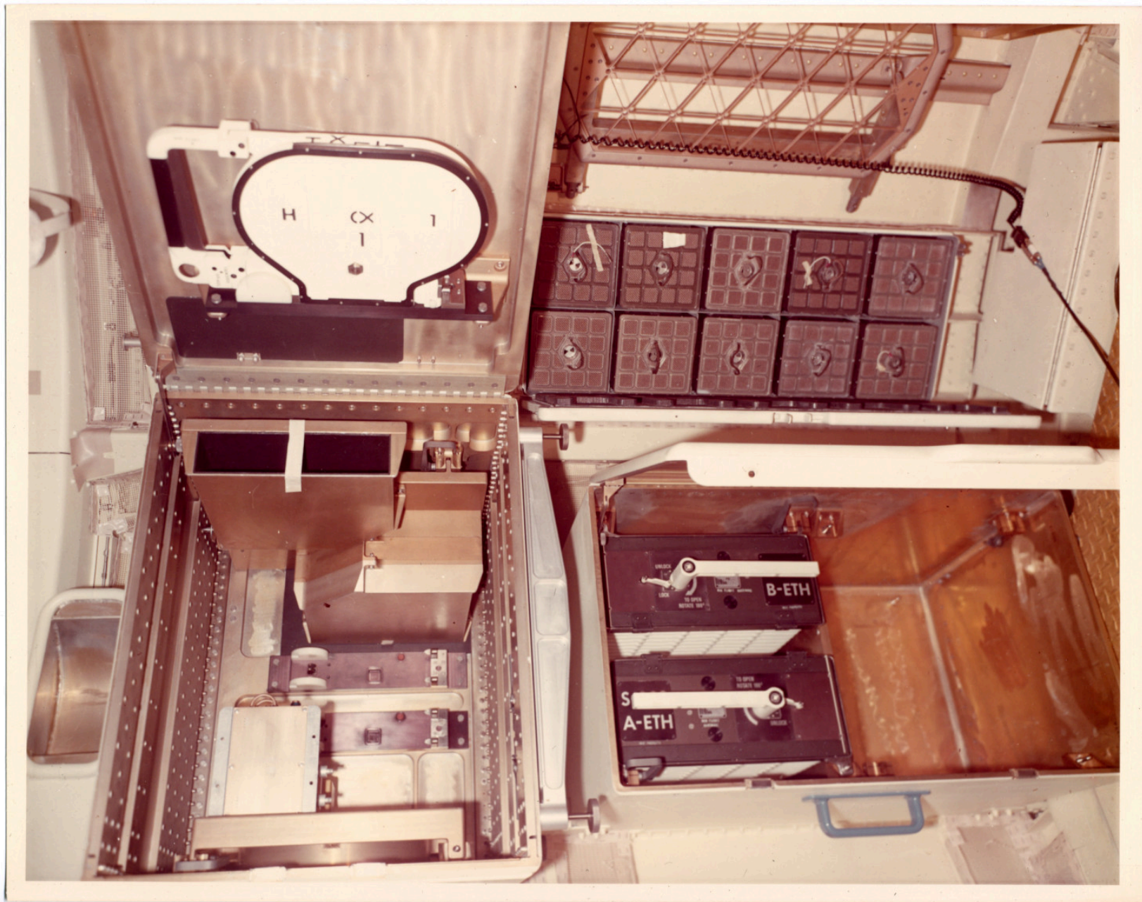
There is a still caption on the back which reads: "FILM VAULTS NO. 1 AND NO. 4, AND CO STOWAGE CONTAINER IN STOWED 2 CONFIGURATION."
