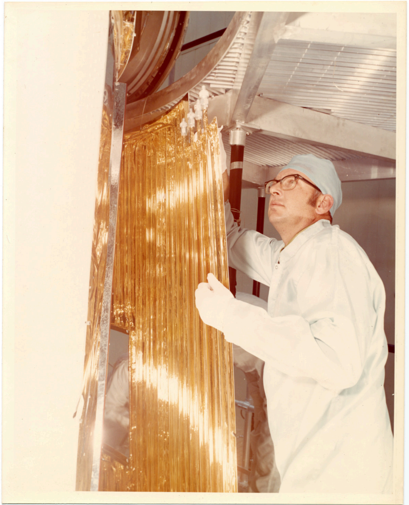
There is a still caption on the back which reads: "FITTING FINAL RADIATOR PANEL INTO PLACE ON MDA FLIGHT ARTICLE. MDA INPUT FOR SEPT 1971."
