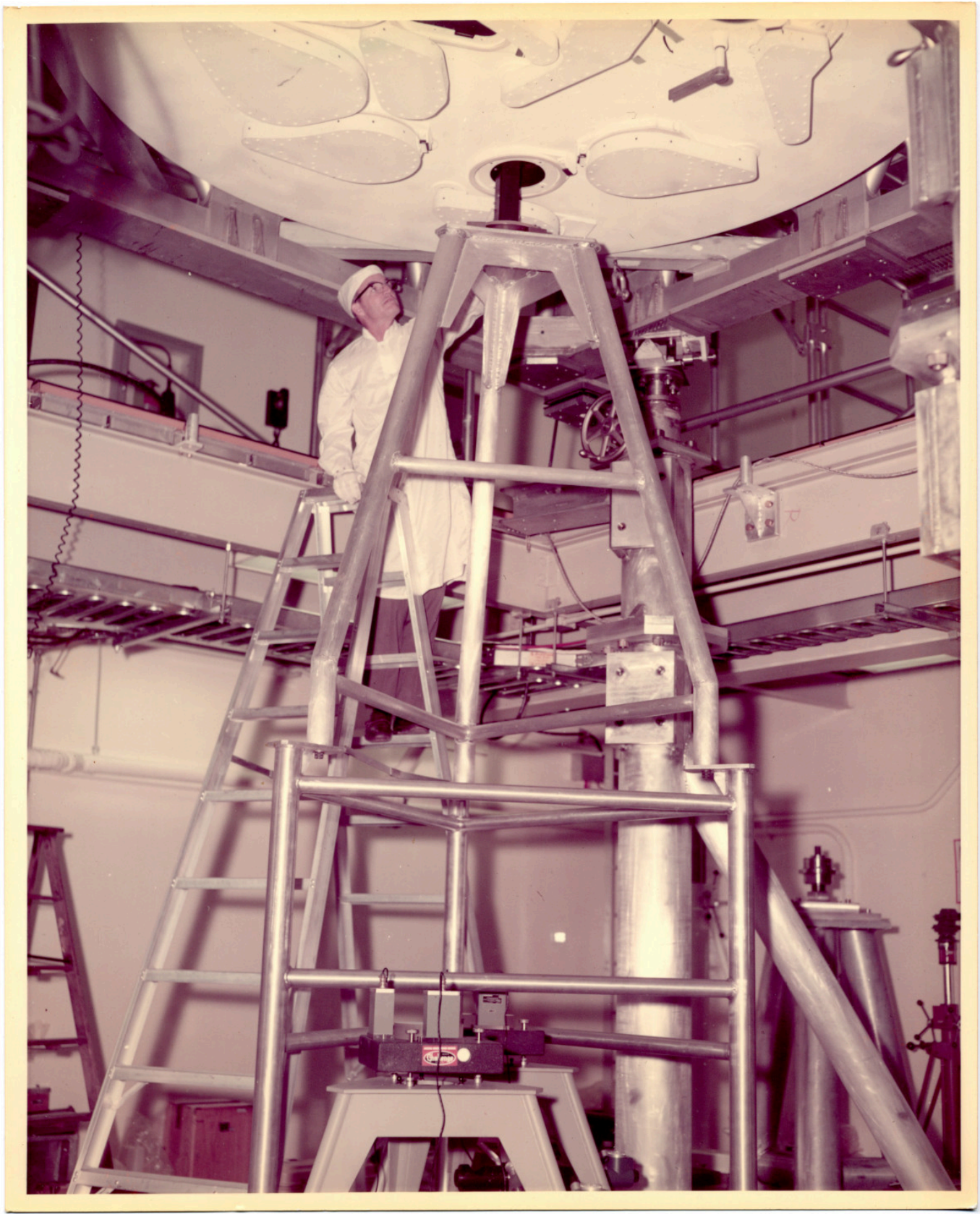
There is a Still Caption on the back that reads, "ATM EXPERIMENT ALIGNMENT TEST, OPTICAL TRANSFER SYSTEM OPERATION."
