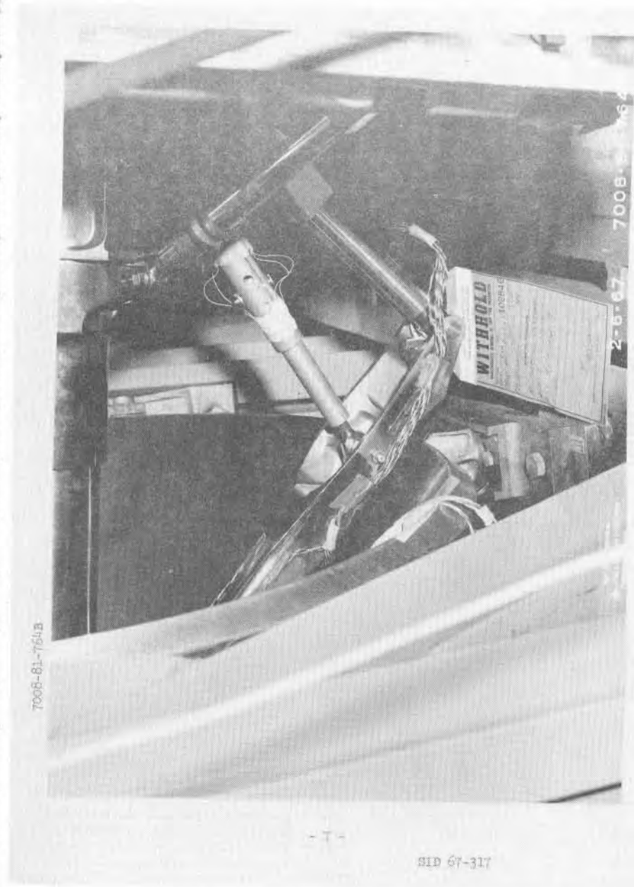
Figure 2. ONE PITCH CONTROL BEAM (A) IN CONTACT WITH DROPLET
