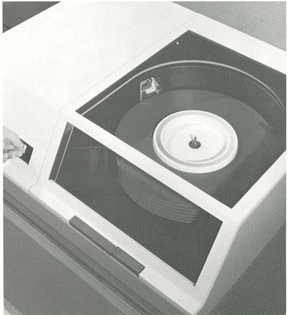
Disc storage unit of IBM 360, Model 40, computer, recently installed at Brown's computer facility. This disc system offers several operating advantages over magnetic tape.
