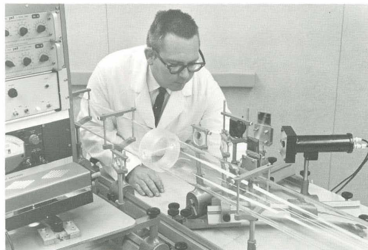
Brilliant red laser beam is shown here providing a probe for precise measurement of liquid velocity without disturbing flow. This is one of the many laser studies being undertaken by Brown's research laboratories.
