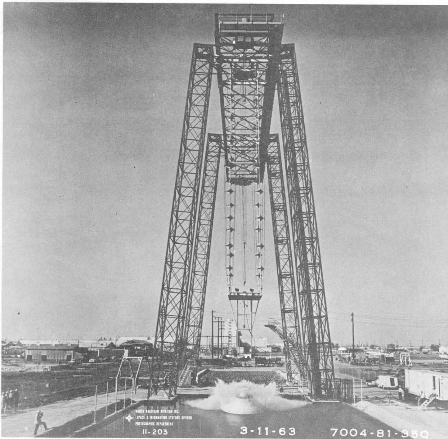
Figure 21. Water Impact Test of "Boilerplate" Apollo
