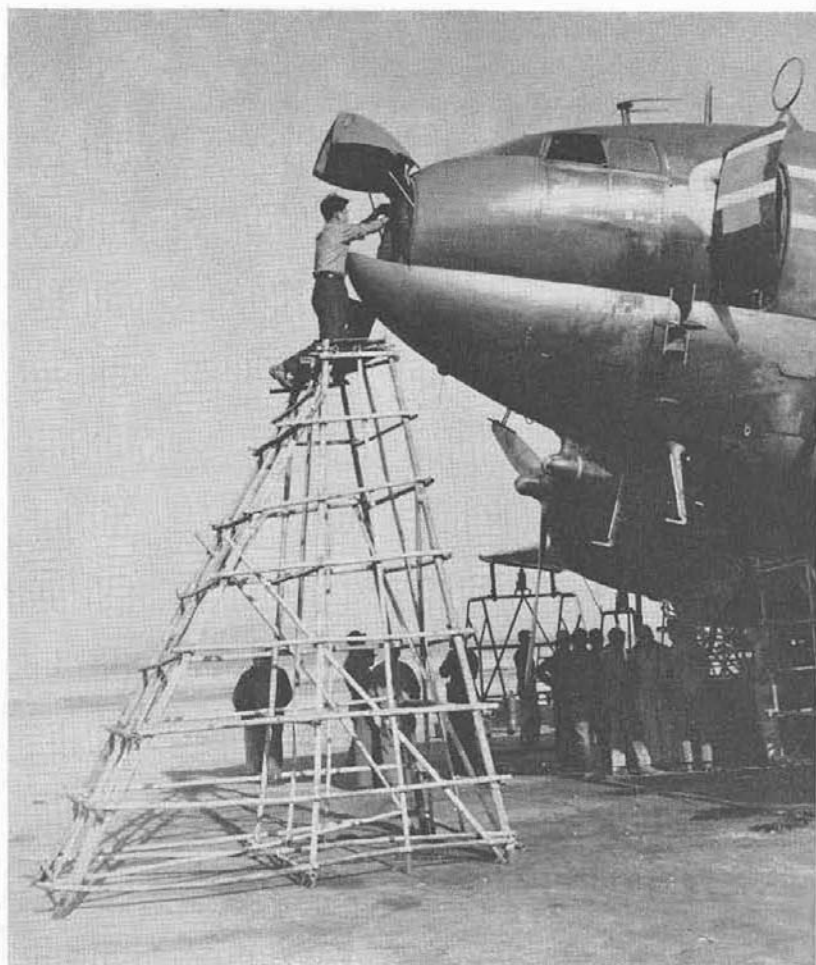
In airline's early days, maintenance stands for its surplus aircraft were fashioned by lashing together bamboo poles.
