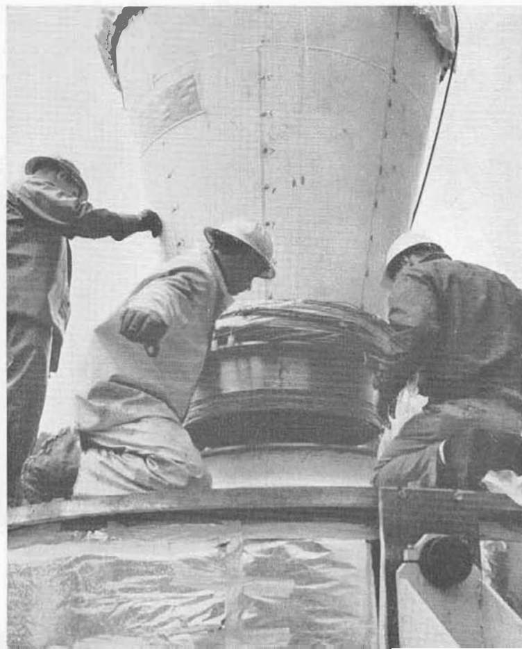
With the aft-closure section already secured to the motor, workmen carefully guide nozzle into position as final step in assembly of the booster.
