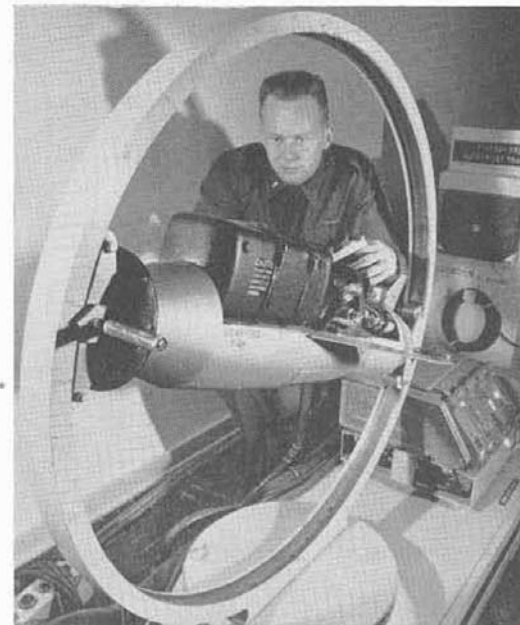
Autopilot training device permits flier to maneuver craft automatically as he would in actual flight.
