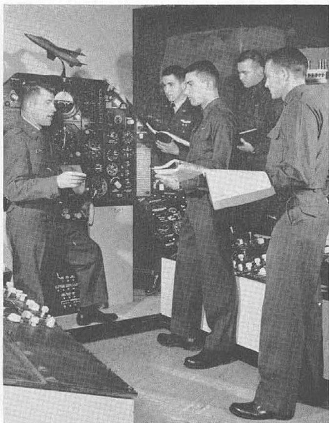
More than twice the size of a normal cockpit in the F-105D, this walk-in version permits group work on familiarization.
