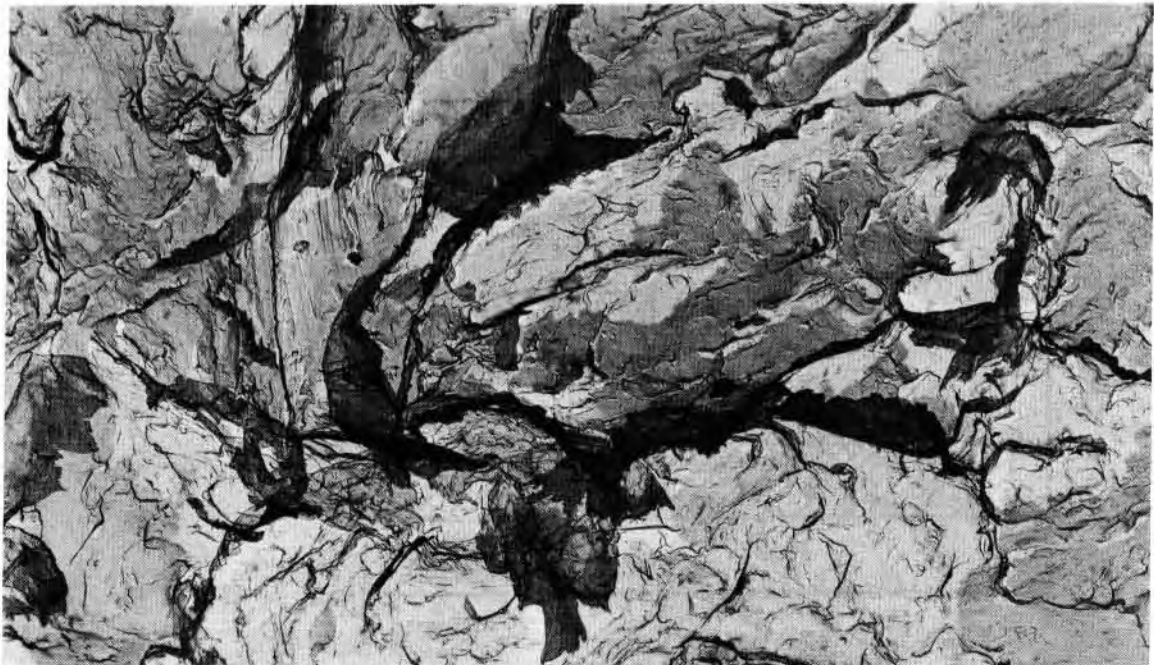
Figure 19. A-302 Notched Girth Weld Heat-Affected Zone Specimen, Tested in 10,000 psi Hydrogen; 10-Day Hold
