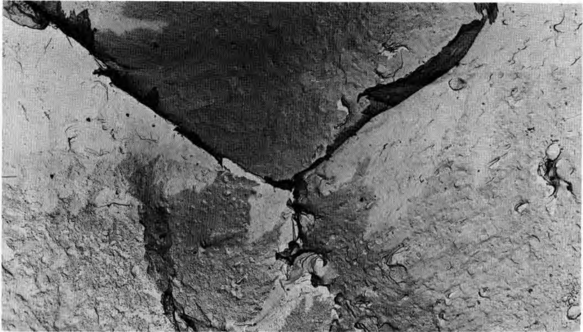
Figure 18. A-302 Notched Longitudinal Weld Metal Specimen Tested in 10,000 psi Hydrogen; 1-Day Hold
