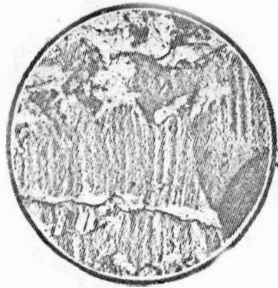
Electron Microscope Fractograph Showing Fatigue Striations 3000X
