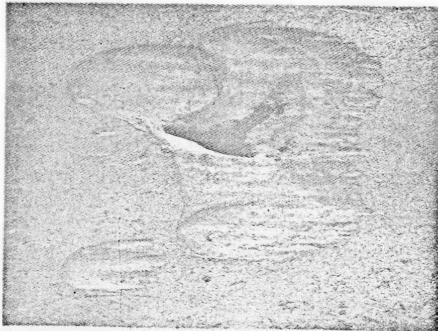
FIGURE 10. A More Advanced Degree of Erosion. Mag: 4X
