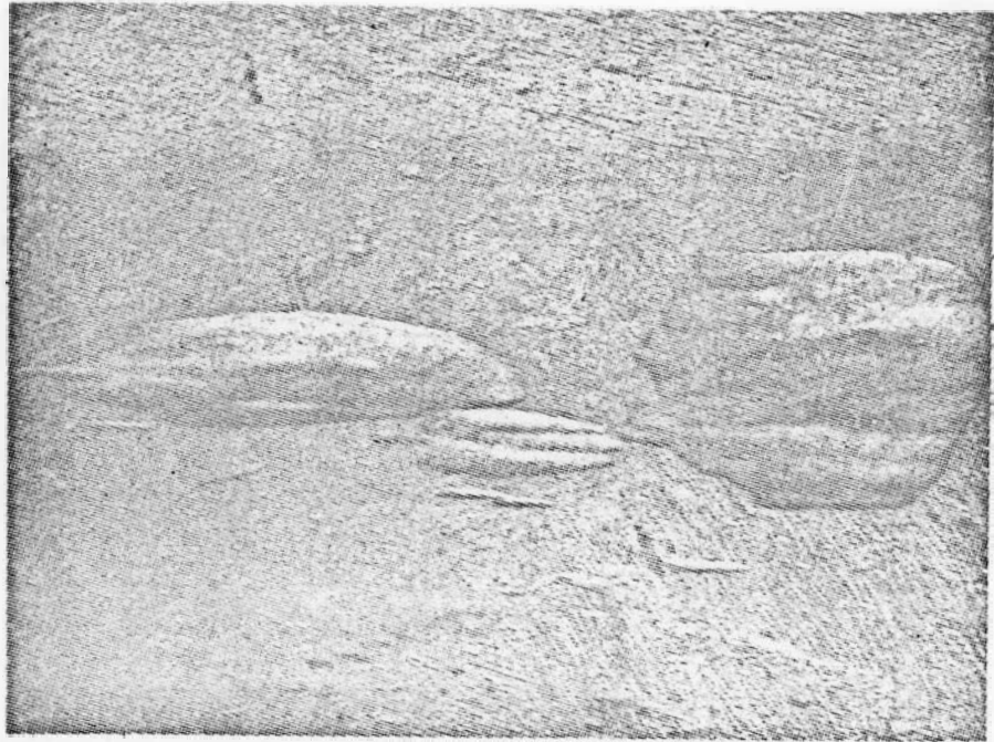
FIGURE 9. Typical Erosion on the Combustion Side of the Shingle. Mag: 4X
