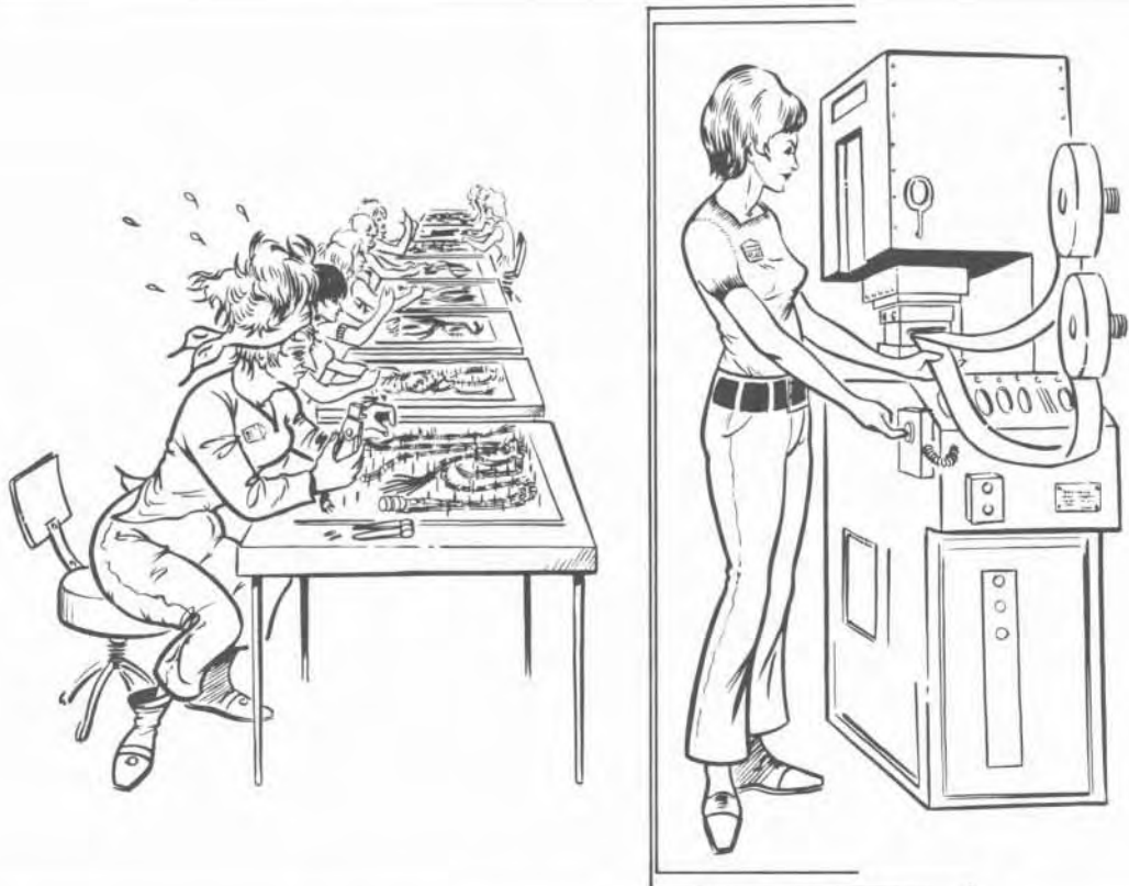
Figure 5. Pictorial Presentation of Comparison Between Methods for Round-Wire and Flat-Cable Harness Assembly (2)
