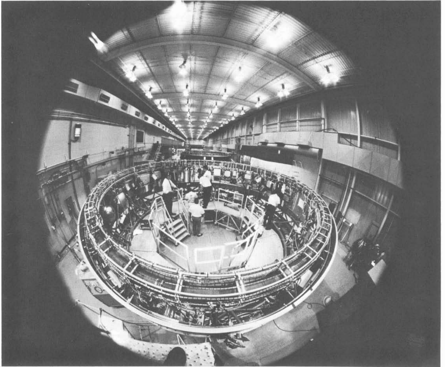
Instrument unit—the flight control center for the Saturn.
