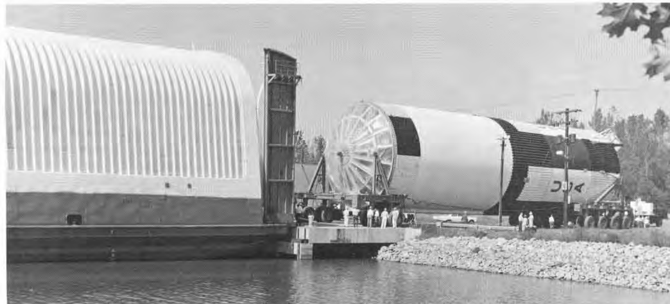
A ground test Saturn V booster rolls out of the cargo hangar of the new NASA barge "Poseidon."
