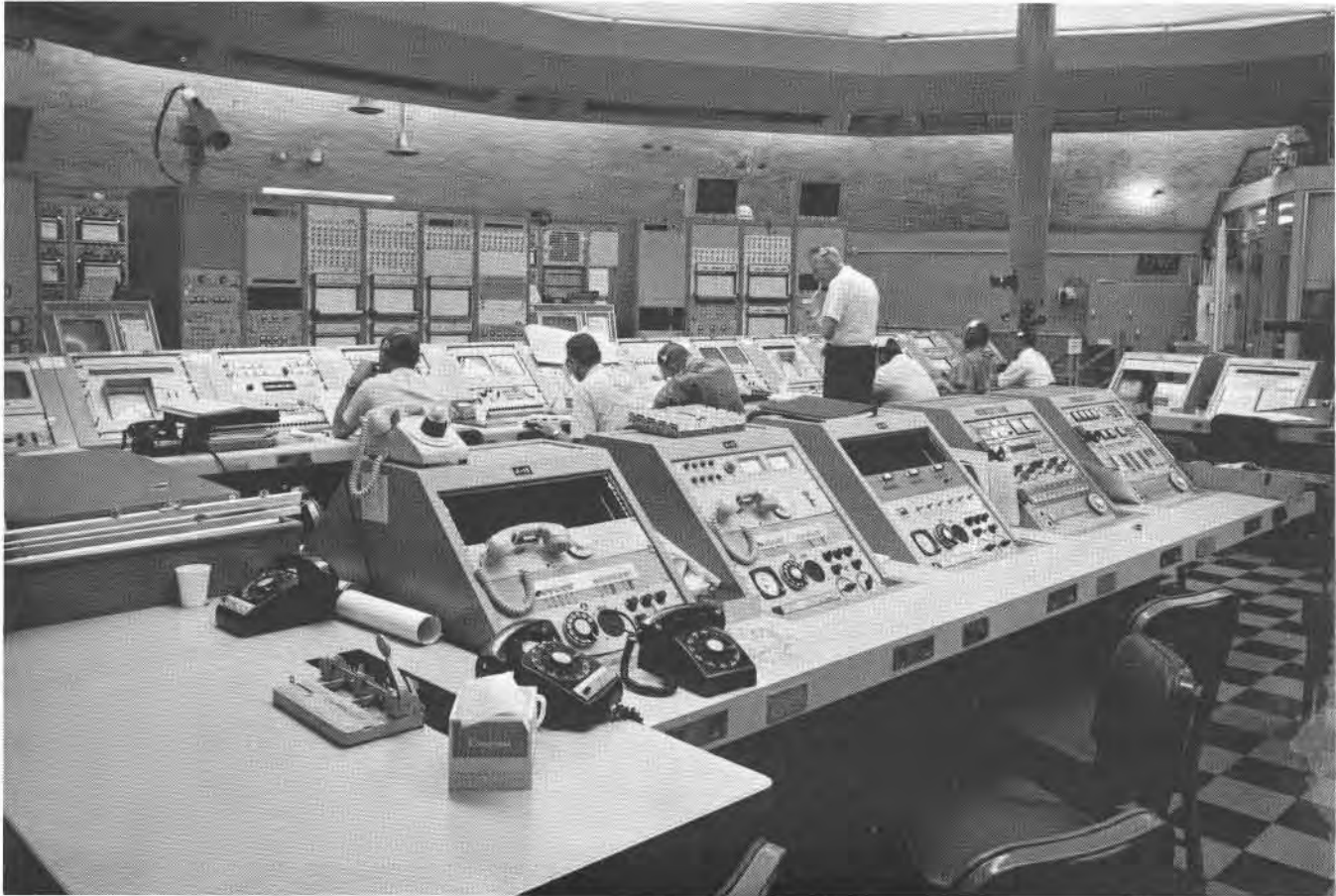
Engineers and technicians at consoles of launch control center conduct test and checkout operations prior to launch of Saturn 1B.
