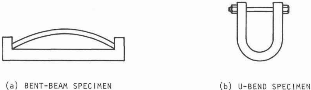
Figure 12. Bent-Beam and U-Bend Specimens
