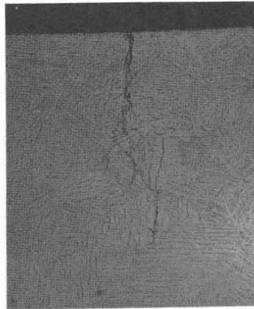
Stress-Corrosion Cracking (Ti-5Al-2.5Sn)
