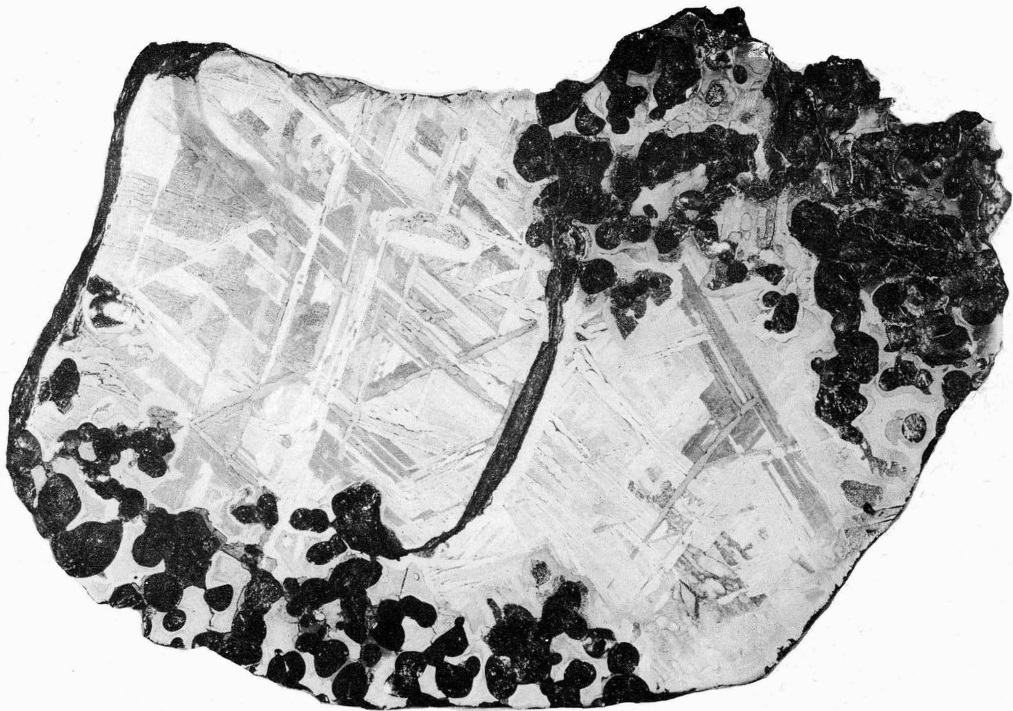
Fig. 4 A slice of the Brenham, Kansas, stony-iron meteorite, a pallasite. Note Widmanstätten pattern juxtaposed with iron mesh whose interstices are filled with glassy-silica olivine. Natural size. (Smithsonian Institution photograph.)
