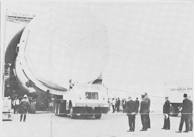
S-II TRANSPORT — The S-II-10, second stage of the Saturn V launch vehicle, shown as it left Seal Beach last month. The Division-built stage is now in a test stand at NASA's Mississippi Test Facility, being readied for static test firing Aug. 28. The S-II-9 was successfully static test fired on June 20 at NASA's MTF.
