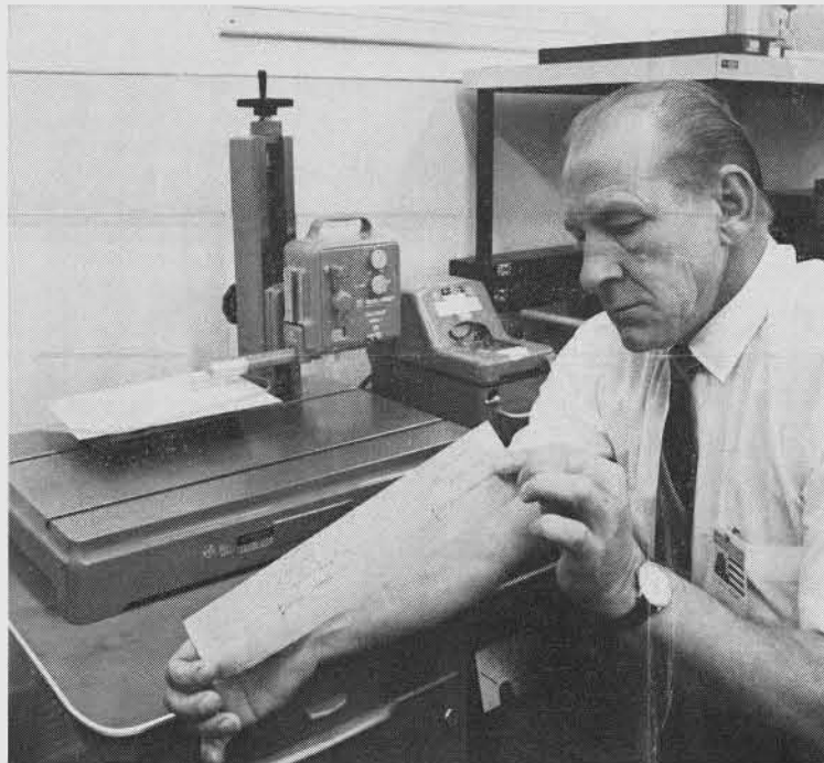
MICROINCH MARKINGS — Joeschke examines readout from machine with stylus so sensitive it can measure in microinches any scratches on a spacecraft window. Hair is 3,000 microinches.
