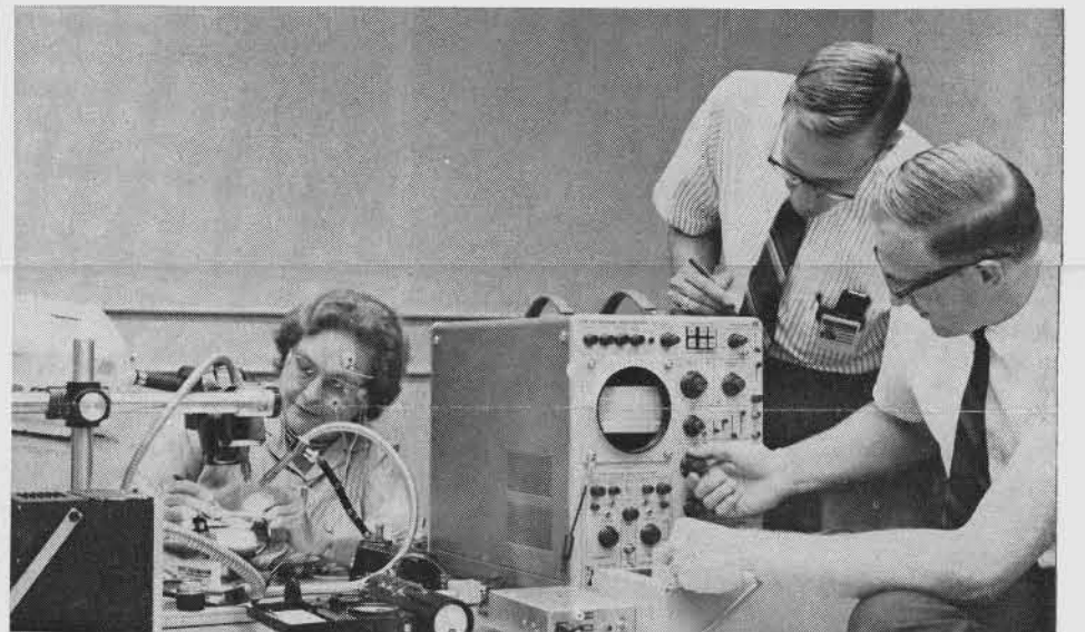
MICROSCOPIC PHOTOGRAPHY — Jerry Theaker, technical photographer, left, foreground, synchronizes equipment for filming the micro assembly. Beulah Abbott, Dept. 324, sets up assembly under microscope, as Howard Maples, manufacturing engineer, Autonetics Dept. 33, takes notes. Above, Theaker bore-sights movie camera to align it with Beulah's microscope.
