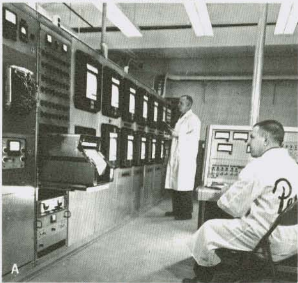
(A) Remote control center is connected to self-contained test cells. This equipment can record 75 separate pieces of information at the same time. (B) The Pesco Cryogenics Laboratory in Perry, Ohio. (C) A hydrogen booster pump installed for testing in Pesco's 7000-gallon dewar. (D) Dudley Rose, Pesco Cryogenics Laboratory manager.
