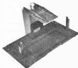
ST-124M-3 PLATFORM ELECTRONIC FIXTURE ASSEMBLY
