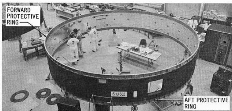
7. FORWARD AND AFT PROTECTIVE RINGS INSTALLED
