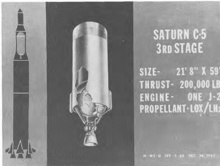
FIGURE 92. S-IVB STAGE CUTAWAY
