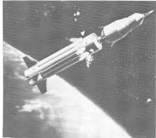
FIGURE 50. SEPARATION OF UPPER STAGES FROM BOOSTER
