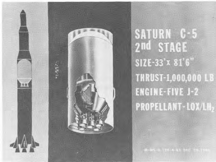
FIGURE 87. S-II STAGE CUTAWAY
