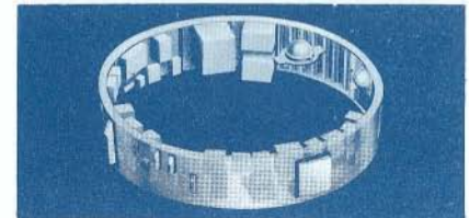
Block II Instrument Units. The simplification of systems reduced weight markedly in the later version.
