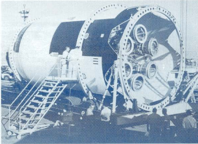
Douglas Aircraft Company engineers check out S-IV stage at their Santa Monica plant.
