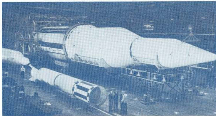
A completed early Saturn, "horizontally mated," seen next to a Redstone and a Jupiter vehicle.
