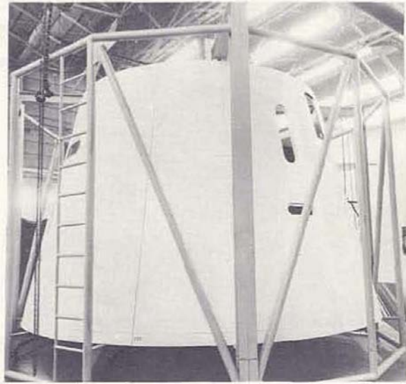
FIGURE 56. FORWARD INTERSTAGE MOCKUP
