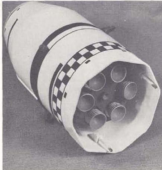
FIGURE 41. SIX-ENGINE CONFIGURATION OF THE S-IV STAGE
