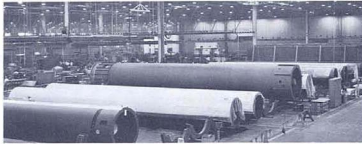
LOX AND FUEL TANKS READY FOR CLUSTERING
