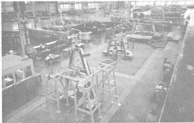
Figure III-11 - Engine Fairing Tooling at Michoud
