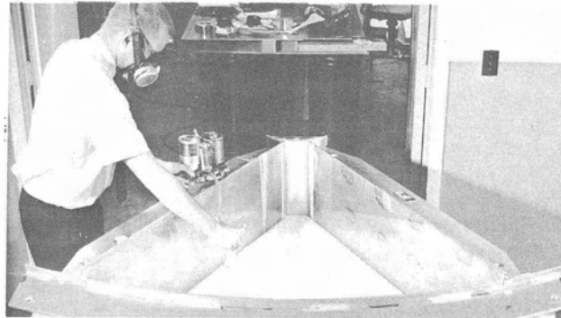
Figure X-10 - A Hygienist Takes a Sample of Toxic Polyurethane Resin Vapors to Determine Their Concentration
