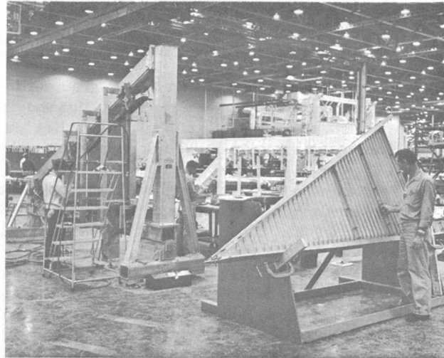
Figure IX-5 - A Cruciform Baffle Segment is in its Assembly Fixture at the Left. Another Baffle Segment is on a Stand.
