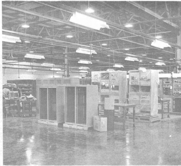
Figure III-18 - GSE/MSE Drawer and Rack Assemblies Shown Nearing Completion and also Ready for Shipment
