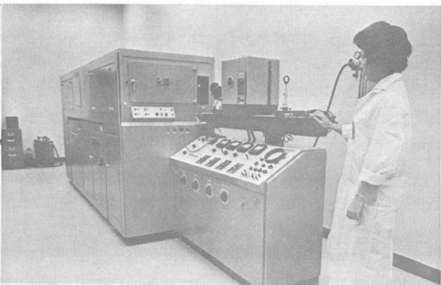
Figure IV-7 - Three-Meter Grating Spectrograph in Quality Evaluation Laboratory
