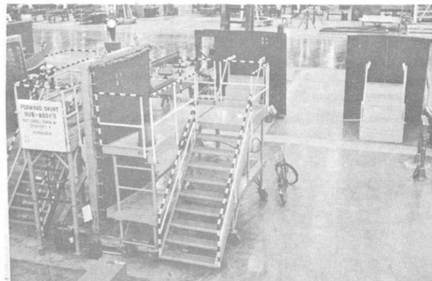
Figure IX-8 - Skin Panels for the S-IC-S are Assembled in the Fixture at the Left and Held for Shipment as shown
