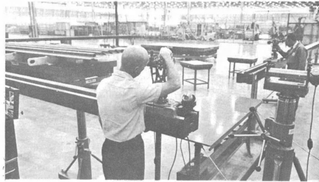
Figure IV-16 - Tooling Bars and Associated Optical Tooling Equipment in Use in Michoud Plant
