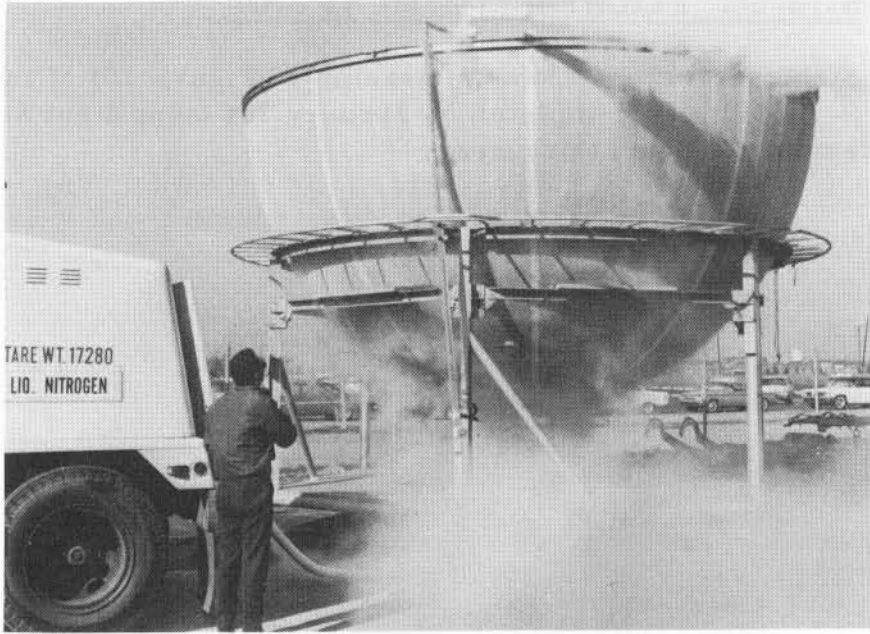
Figure 9 - S-IVB/IU Forward Dome During LN 2 Shock Test
