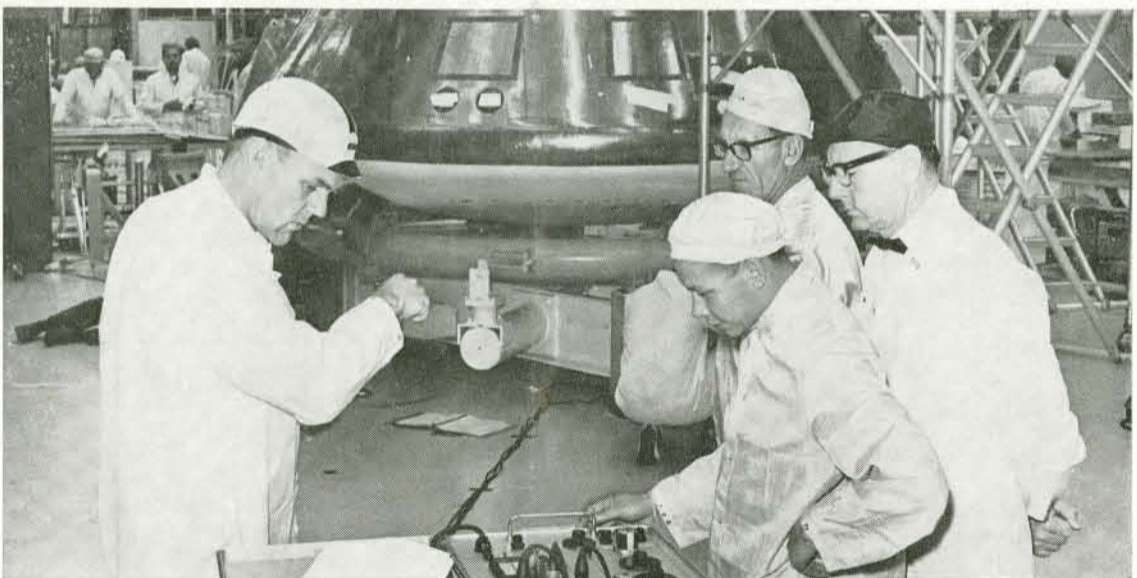
WEIGHT AND BALANCE — One of final checks of command module was weight and balance verification. Shown, from left, are Lloyd Woolover, Harry Takechi, Art Mirandi, Roy Reynolds.
