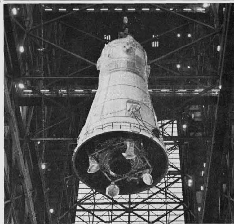
PREPARATIONS — Apollo 10 spacecraft, including division-built command and service modules, spacecraft/lunar module adapter, and lunar module, is hoisted ceiling-ward in preparation for mating with its waiting launch vehicle. Scheduled for launch in May, Apollo 10 will be lunar orbit flight designed to check out lunar module under moon environment conditions.
