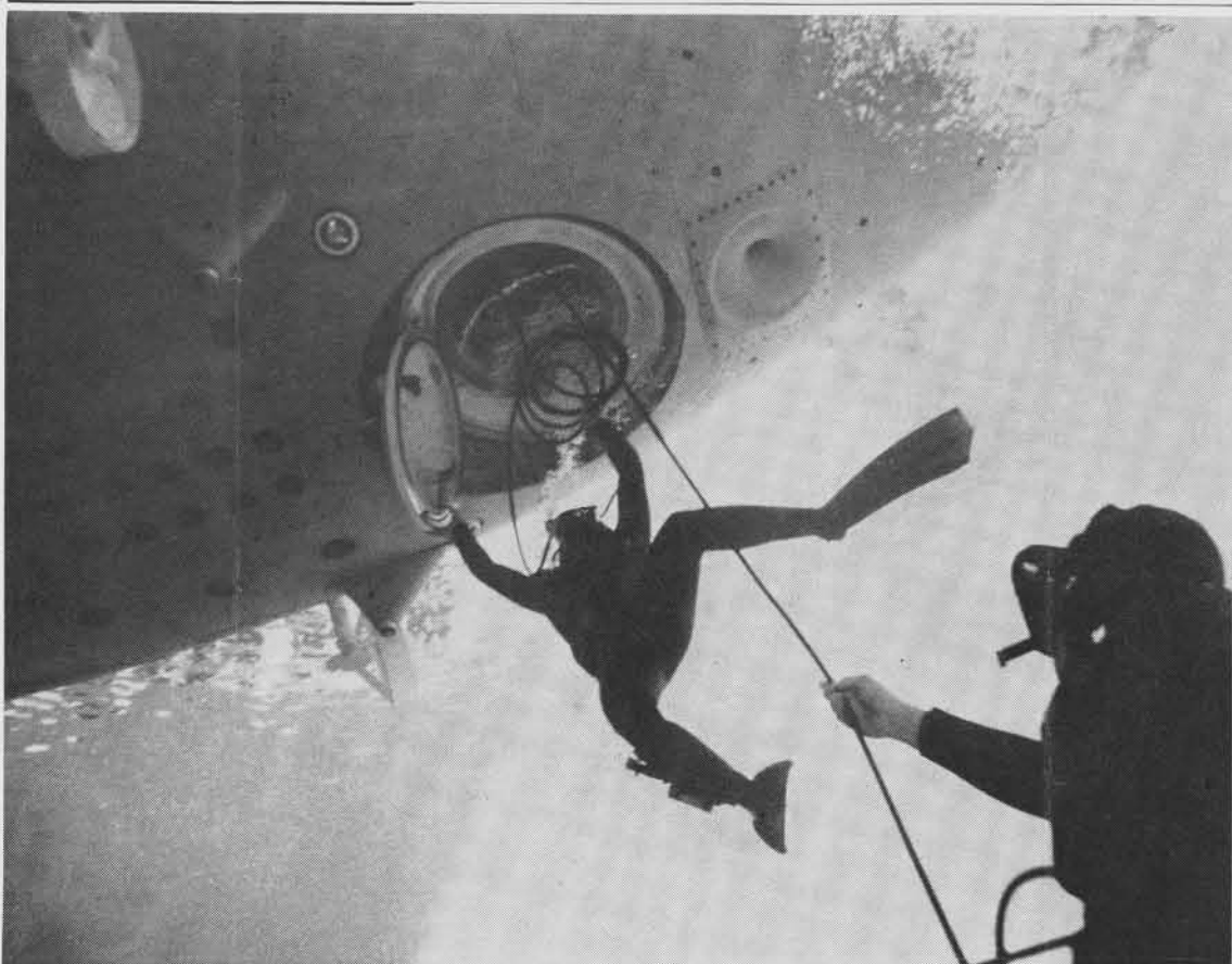
THE ONLY WAY TO GO — Division Ocean Systems Operations divers test lock-out section of Beaver Mark IV in tank submergence test. Diver lock out is one of key features of Beaver submersible, now undergoing sea trials at Catalina Island that are scheduled for completion in early spring.
