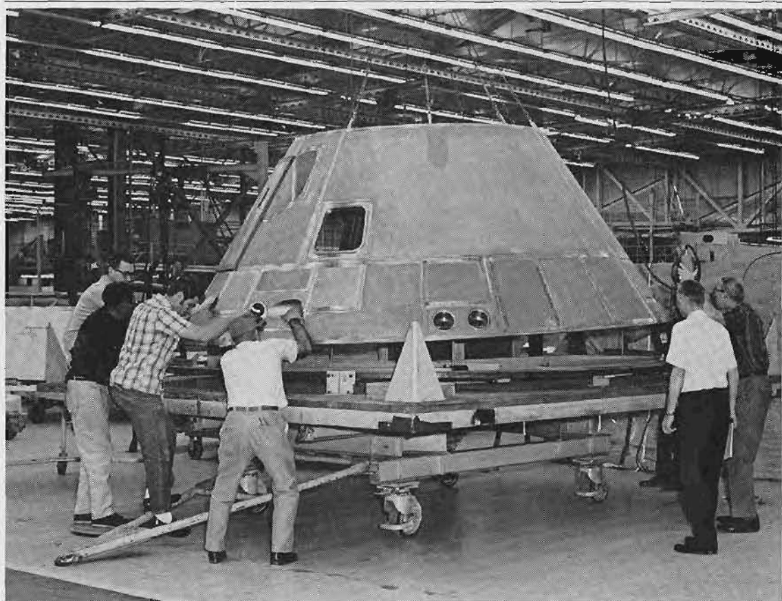
READY TO GO — Employees in Apollo Structures Assembly carefully lower forward heat shield section for Apollo Spacecraft 118 onto dolly for shipment to Avco Corp. where ablative material will be added. Department Heat Shield team reduced fabrication time on heat shield section by one-half over time taken on same component at start of Apollo Block II program.
