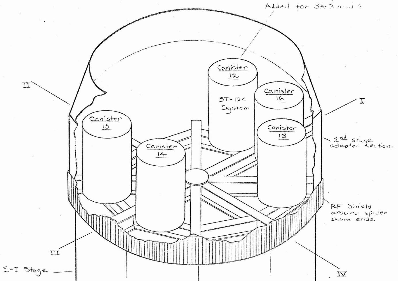
Major Electrical Components Located In Pressurized Canisters
