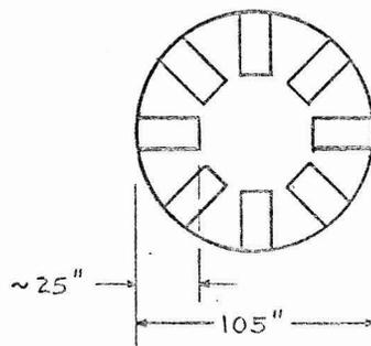
Baffle weight added for SA-2, 3 & 4  $\sim 300$  lbs.
