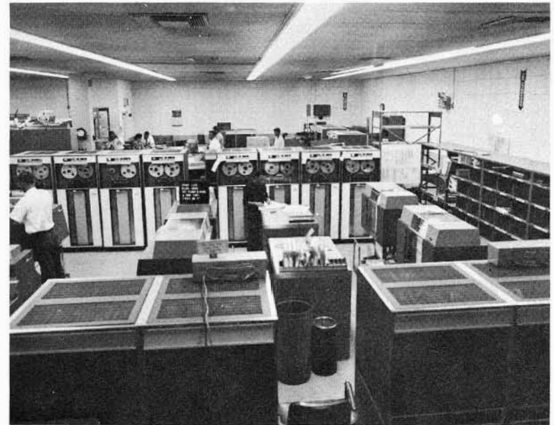
1401 COMPUTERS FOR PREPARATION OF INPUT DATA FOR 7094 COMPUTER AND CONVERSION OF MAGNETIC TAPE DATA TO HARD COPY OR CARD FORM
