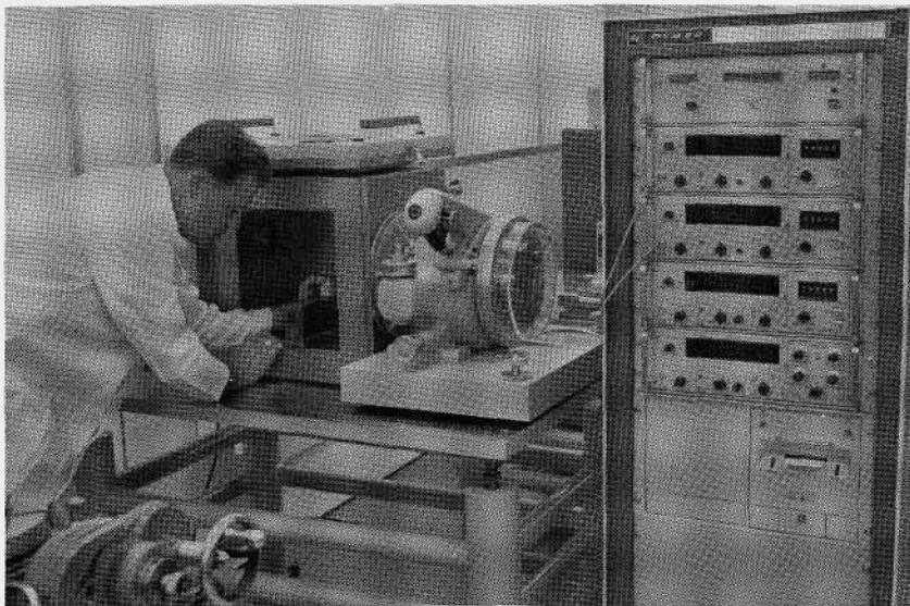
Vinco Dividing Head with Temperature Chamber and Accelerometer Test Console
