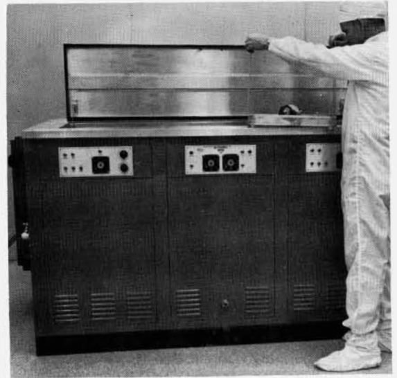
Ultrasonic Cleaning Operation
