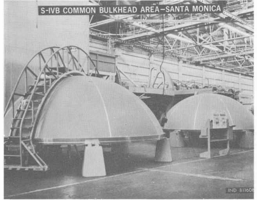
S-IVB BONDING HONEYCOMB TO AFT DOME SANTA MONICA
