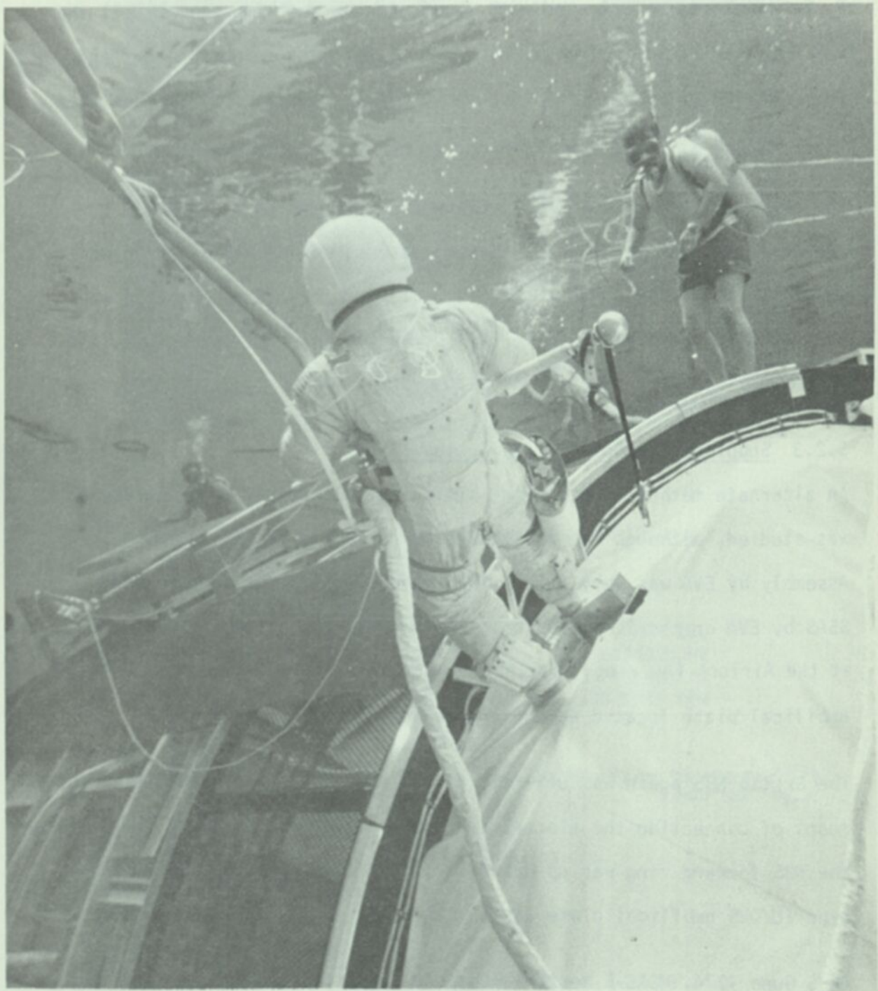
FIGURE 5-39 ASTRONAUT TETHERED AT DISCONE ANTENNA BOOM USING FIVE SAIL POLE SEGMENTS WITH CABLE CUTTERS ATTACHED TO CUT DEBRIS STRAP
